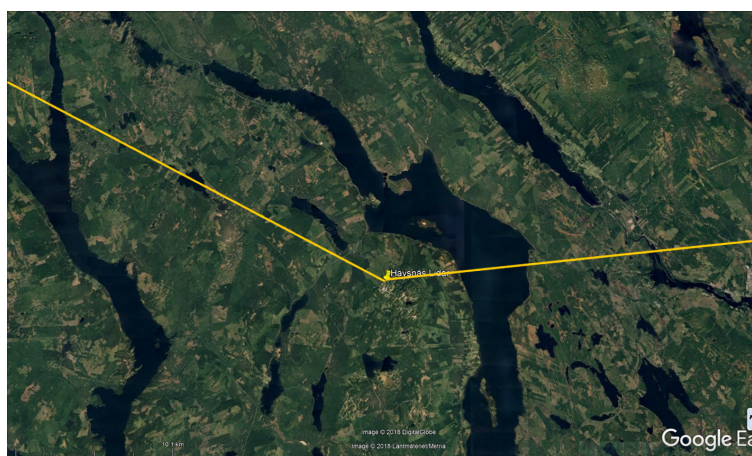
Figure 2-8. Location of Lidar at Havsnäs Wind Farm and surroundings. The wind direction sector 297° to 85° (representing patchy forest and lakes) was used in the analysis. The sector (free from turbine wakes and tower shadows) is indicated by yellow lines.
