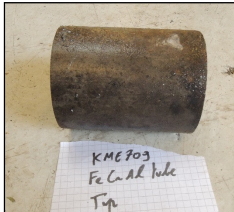
Figure 11. Tip of the FeCrAl tube after cut for analysis
