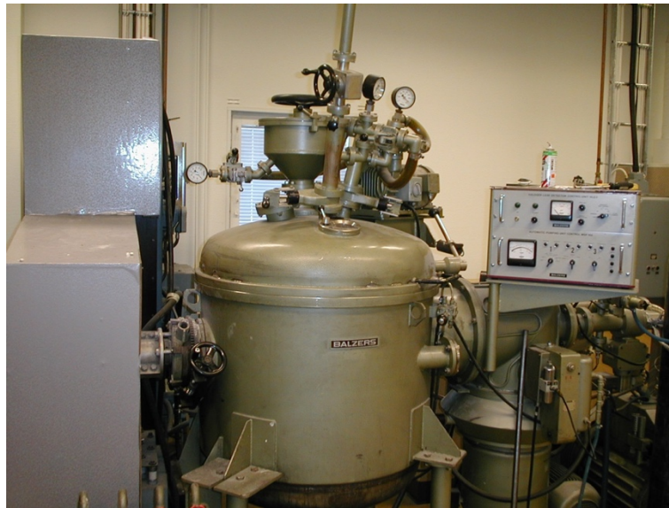
Figure 5: Induction furnace used in the production of the lab-melts at Kanthal.
