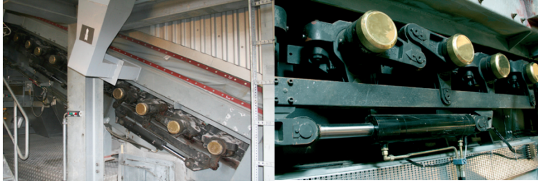
Figure 3: Photos showing details of the air-cooled grate [10]
