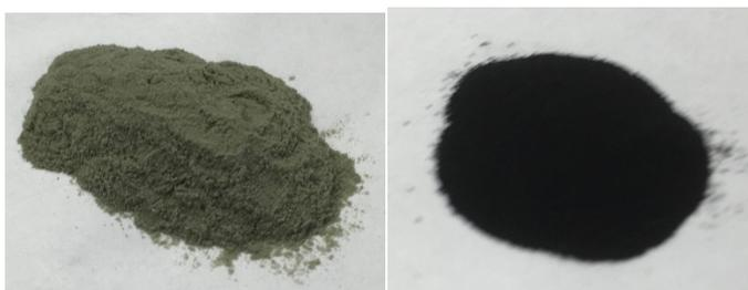
**Figure 20** the Ni-based catalyst before and after calcination and reduction.
