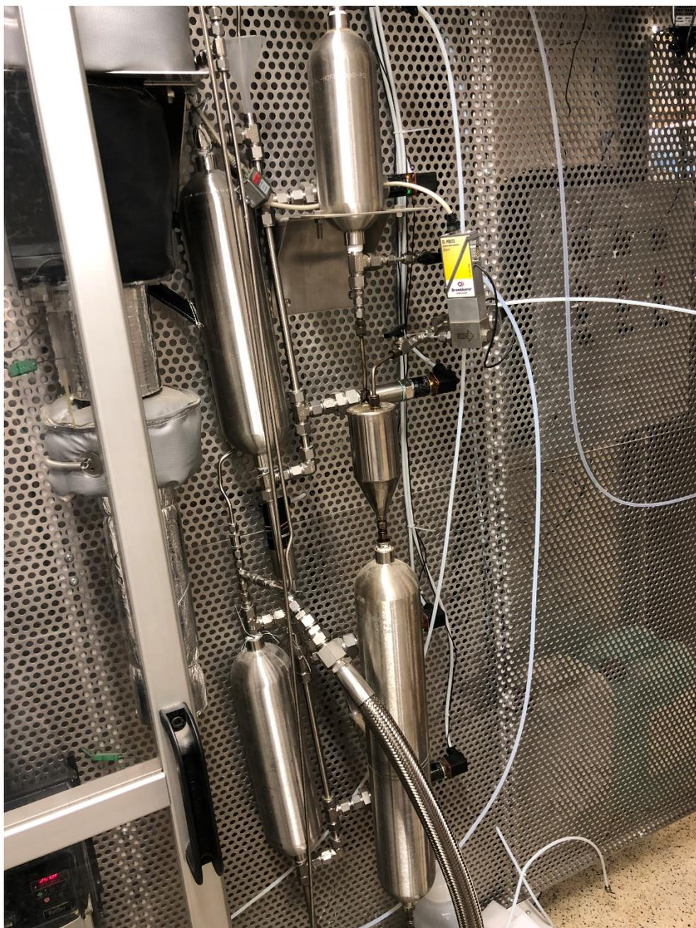
**Figure 10** The compressor vessels and propane/water separator.
