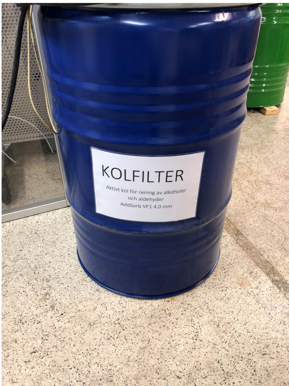
**Figure 13** Activated carbon filter.
