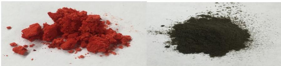
**Figure 19** The Ru-catalyst before and after calcination.
