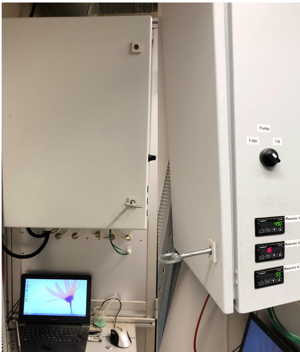
Figure 12 The control computer and electrical cabinet with slave controllers.
