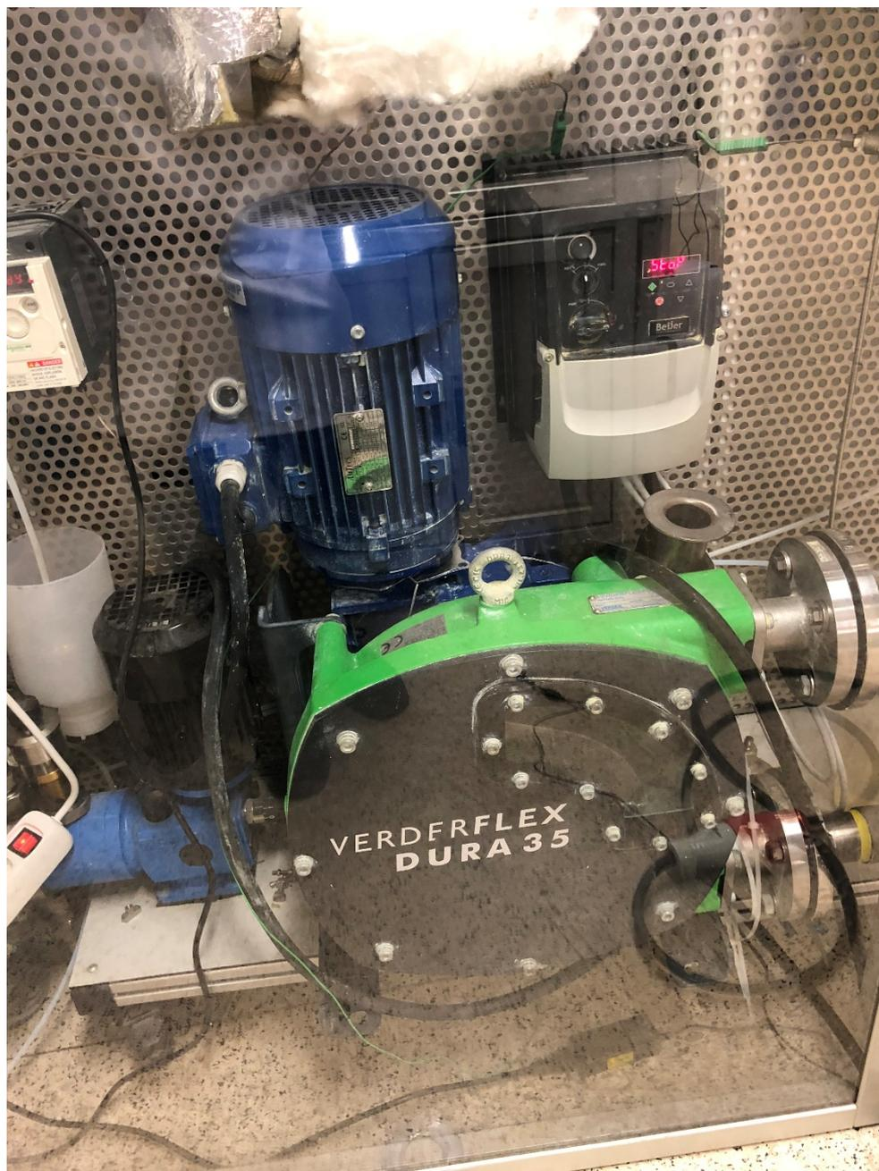
Figure 11 The pump used for creating the recompression pressure in the system.
