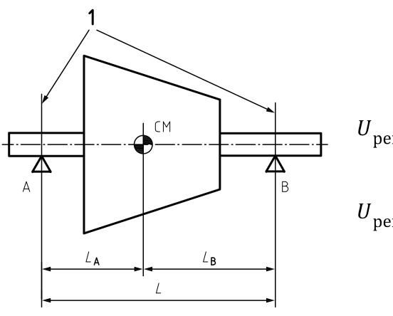
$$U_{\text{per A}} = U_{\text{per }} \frac{L_{\text{B}}}{L}$$
