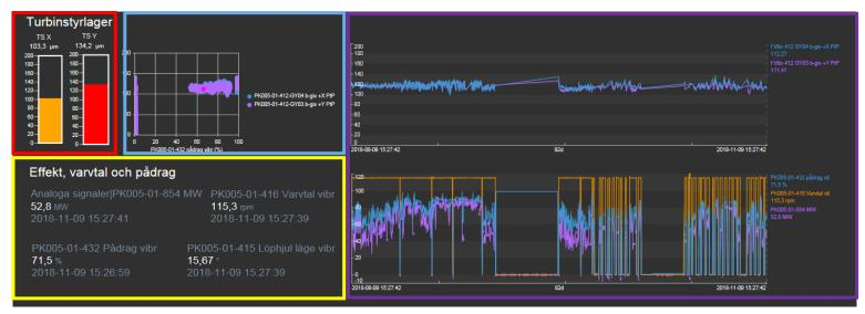
Red box – Present shaft displacement (X and Y direction) Yellow box – Present "production" properties Blue box – Shaft displacement as a function of guide vane opening Purple box – Shaft displacement for the last 3 month (at "stable" operation)
