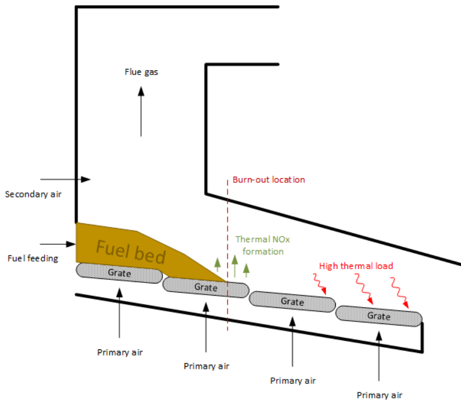
Figure 1. Illustration of exposed grate with insufficient fuel.
