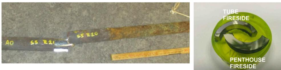
Figure 11: Tube examined for TP347H FG where section consists of both penthouse exposure and boiler exposure
