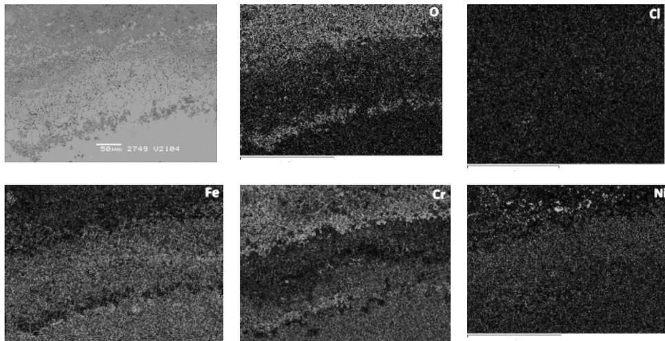
Figure 54: Scanning electron microscopy of corrosion front for Super 304 exposed in boiler E
