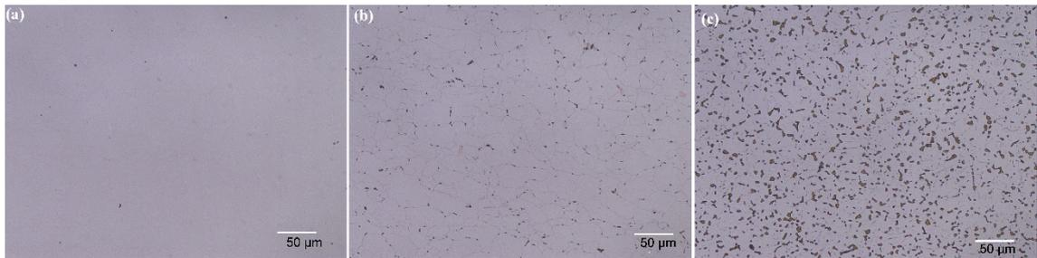
**Figure 46. LOM micrograph of a) as received, b) aged (180° from flue gas), c) aged in flue gas direction (0°). The samples are etched electrolytically with 10% KOH in water**
