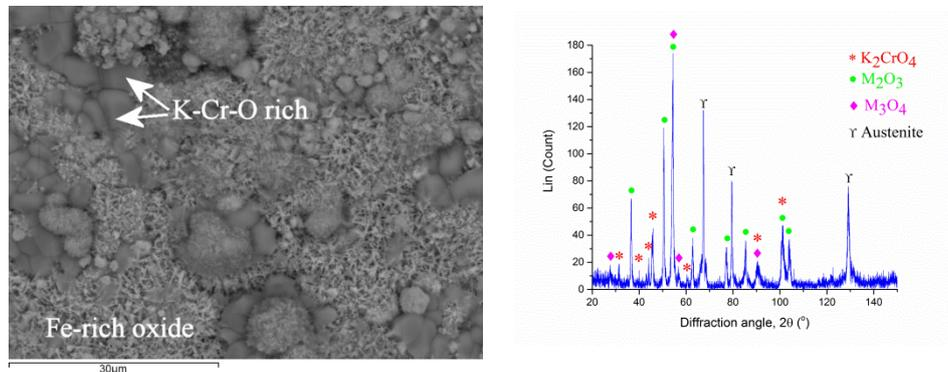
**Figure 49. a) Top view of aged sample in the flue gas direction ( $0^\circ$ ) covered with KCl and exposed 5 % (v/v)  $O_2$  (g) +15 % (v/v)  $H_2O$  (g) +  $N_2$  (g) (balance) atmosphere and b) corresponding XRD analysis**
