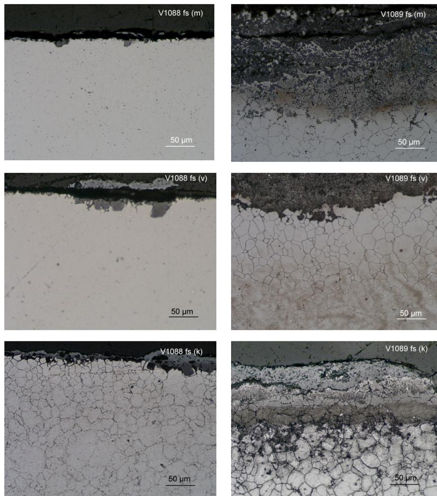
**Figure 56: Use of etchants revealing microstructure 347H from penthouse and within the boiler. the lefthand side is from the penthouse and the right-hand side from within the boiler**
