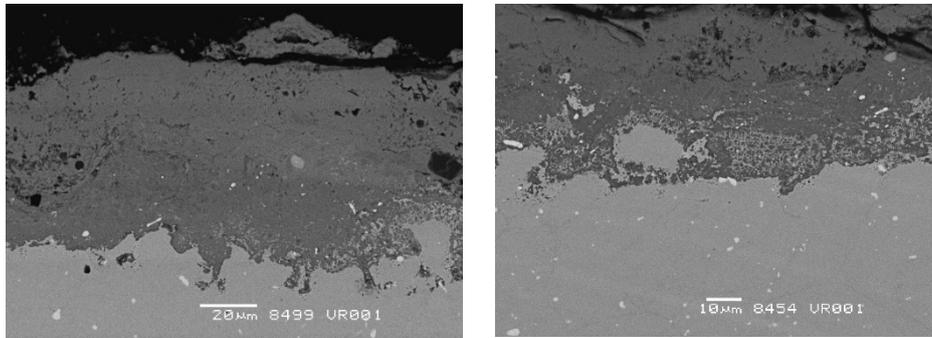
Figure 52: Morphology of fireside oxide on Specimen D
