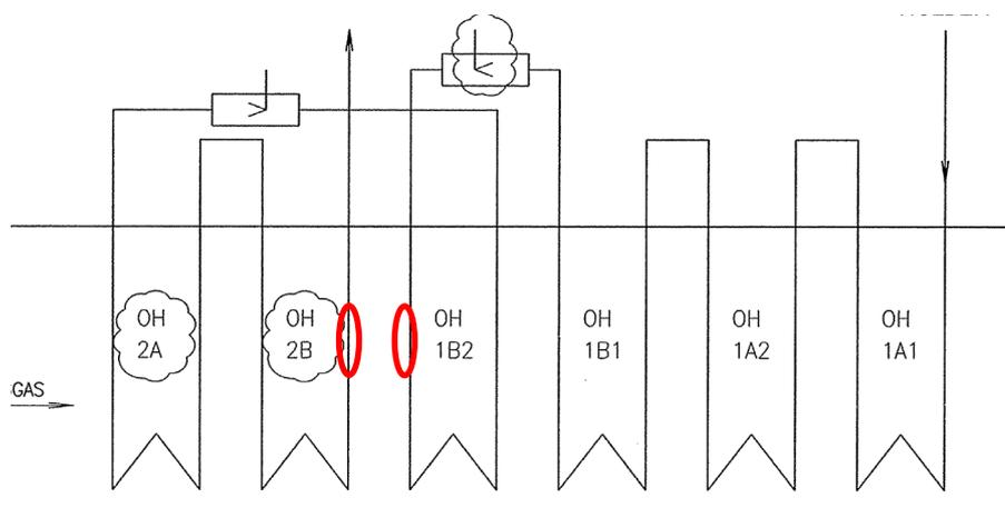
Figure 8. Test materials welded into the superheaters 2B and 1B2 of MEC Waste-to-Energy boiler K1 (Rec)
