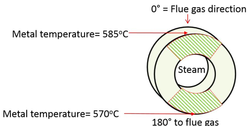
**Figure 10: Locations of 0° and 180° aged samples, and sections used for corrosion testing.**
