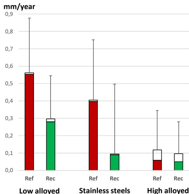
**Figure 40** The filled bars denote the mean corrosion rate of fixed installed superheater test materials in mm/years. The entire bars denote the corrosion rate when all measurements with apparent material growth was discarded. The top error bar reading denotes the mean value of the max corrosion rate per ring.
