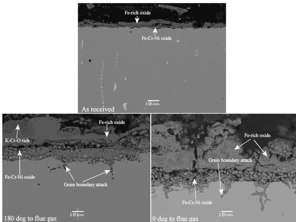
Figure 47. Back scattered images of a) as-received, b) aged sample 180° from flue gas direction and c) aged sample in the flue gas direction (0°) after covering with KCl and exposing in 5 % (v/v) O<sub>2</sub> (g) +15 % (v/v) H<sub>2</sub>O (g) + N<sub>2</sub> (g) (balance) atmosphere at 600°C for 168h
