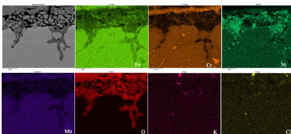
Figure 48. Back scattered SEM image of the 0° aged sample covered with KCl after corrosion exposure in 5 % (v/v) O<sub>2</sub> (g) +15 % (v/v) H<sub>2</sub>O (g) + N<sub>2</sub> (g) (balance) atmosphere at 600°C for 168h
