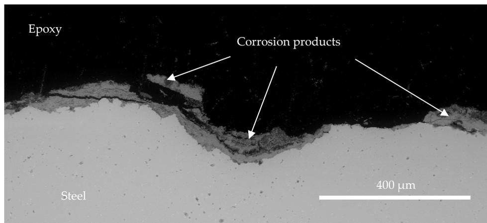
**Figure 27:** BSE image showing a high mag cross section of the flue gas side of 347 Rec Ref at 525 °C for 2000h.
