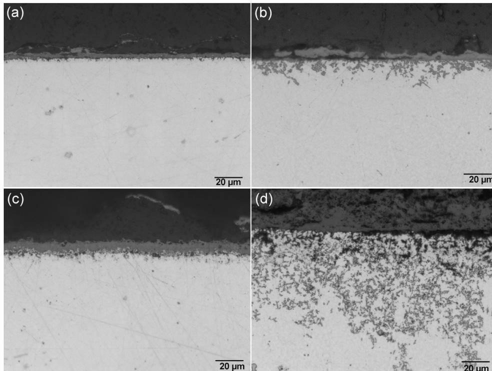
**Figure 44. RLM micrographs after exposure in a 15 % (v/v) H<sub>2</sub>O (g) + 5 % (v/v) O<sub>2</sub> (g) + N<sub>2</sub> (g) (balance) atmosphere at 600°C for 168h. (a) as received KCl-free sample (b) heat-treated KCl-free sample (c) as received covered with KCl sample (d) heat-treated covered with KCl sample**
