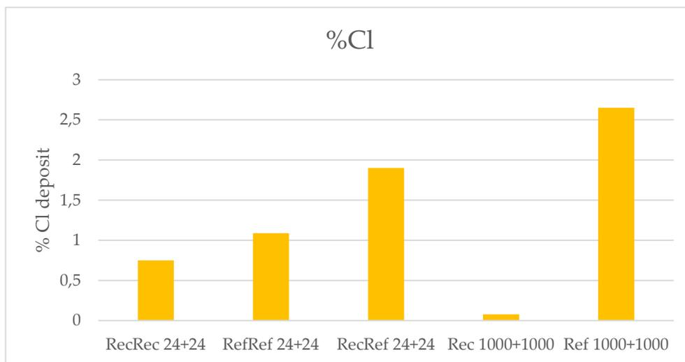
Figure 14. Percentage of chlorine in the different deposits. Line 1 = Rec, Line 2 = Ref.
