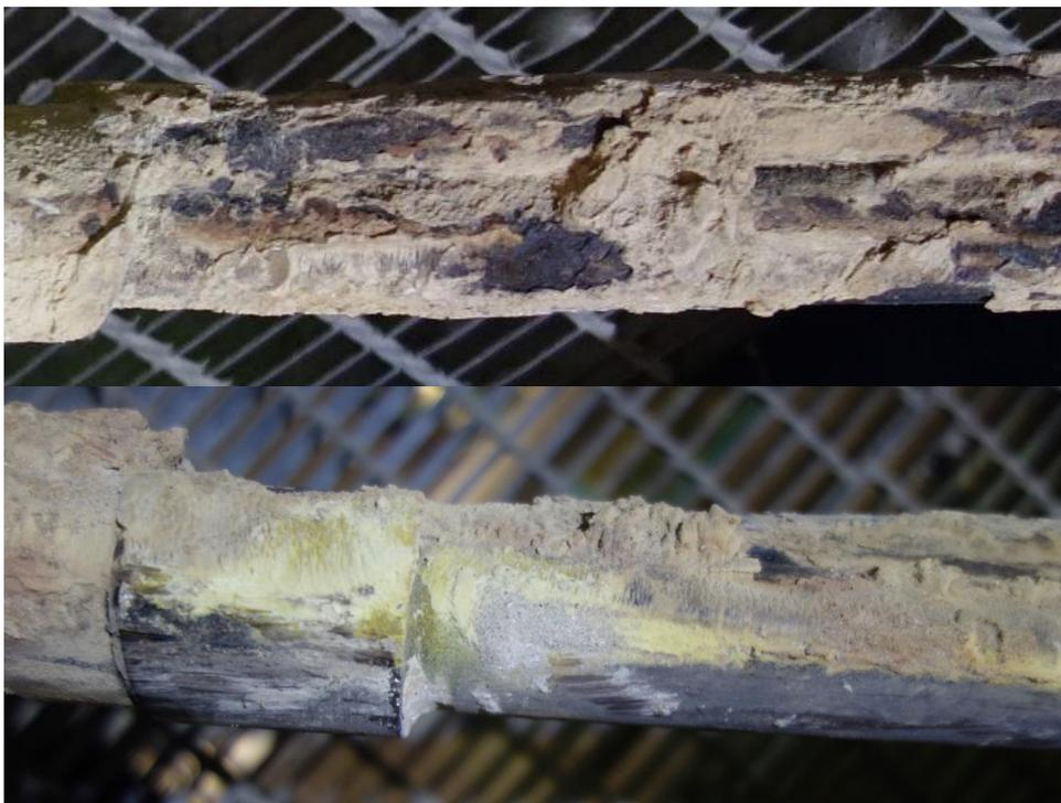
Figure 12. Photographs of the corrosion probes after 1000 + 1000 h Ref (top) and 1000 + 1000 h Rec (lower).
