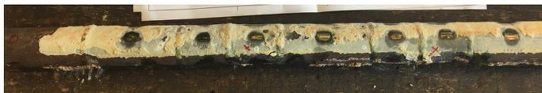
**Figure 16.** Superheater after 6 months in Sulfur Recirculation line
