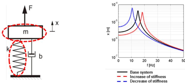
Figure 43 Framework of the system (left figure) and vibration reduction by means of detuning the system (right figure)
