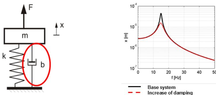
Figure 44 Framework of the system (left figure) and vibration reduction by means of additional damping (right figure)
