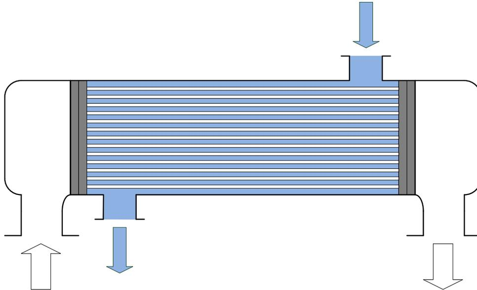
Figure 11 Cross-flow in a heat-exchanger with steam flow (white) and water flow (blue)
