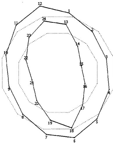
Figure 27 Mode-shape of the stator-core due to magnetic force excitation
