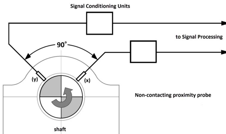
Figure 34 Non-contacting probes for the measurement of relative shaft vibration
