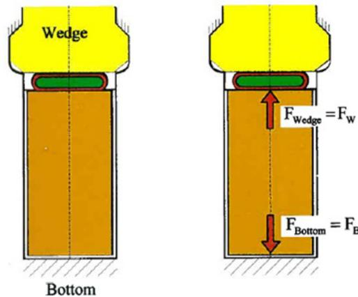
Figure 22 Normal contact forces between copper windings and steel rotor (Nordmann, 2016)
