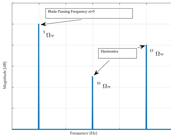
Figure 6 Vibration responses for rotor-stator interaction in the main recirculation pump
