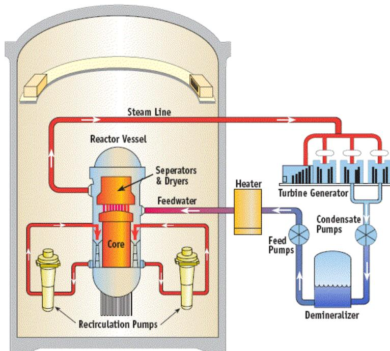
Figure 3 Simplified schematic of a BWR (Commission, 2015)
