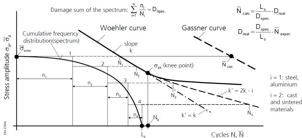
Figure 54 Most commonly used cumulative damage calculation methods
