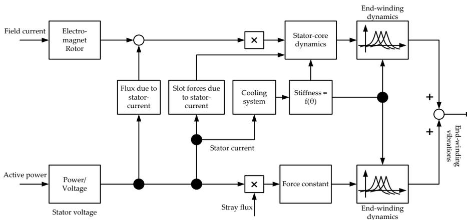
Figure 29 Signal-flow of end-winding vibrations in an electrical synchronous generator
