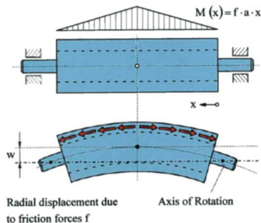
Figure 23 Friction induced bow (bending) in a two pole turbo-generator (Nordmann, 2016)
