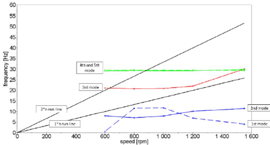
Figure 8 Campbell diagram for a main recirculation pump with fluid bearings
