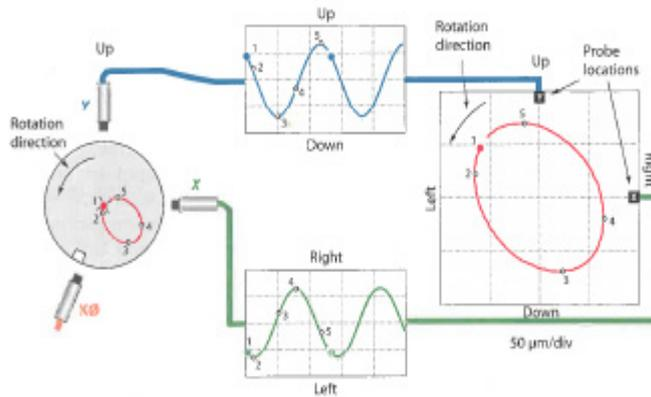
Figure 35 Vibration-orbit of the shaft at one measurement plane generator from vibration signals of two relative vibration sensors
