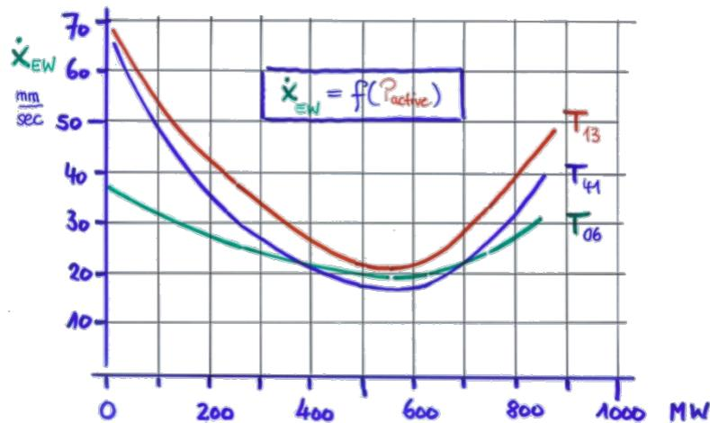
Figure 51 Vibration amplitude versus load diagram for a generator
