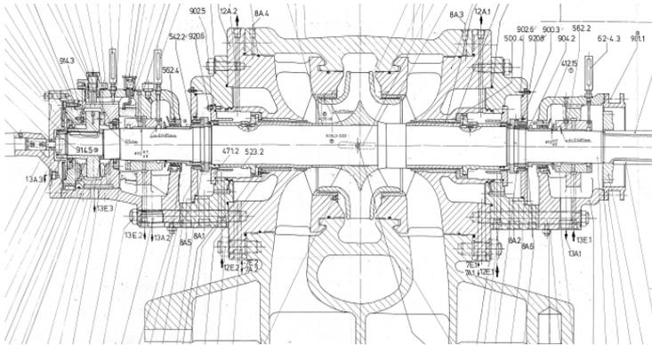
Figure 10 Single-stage, double flow centrifugal feed water pump system
