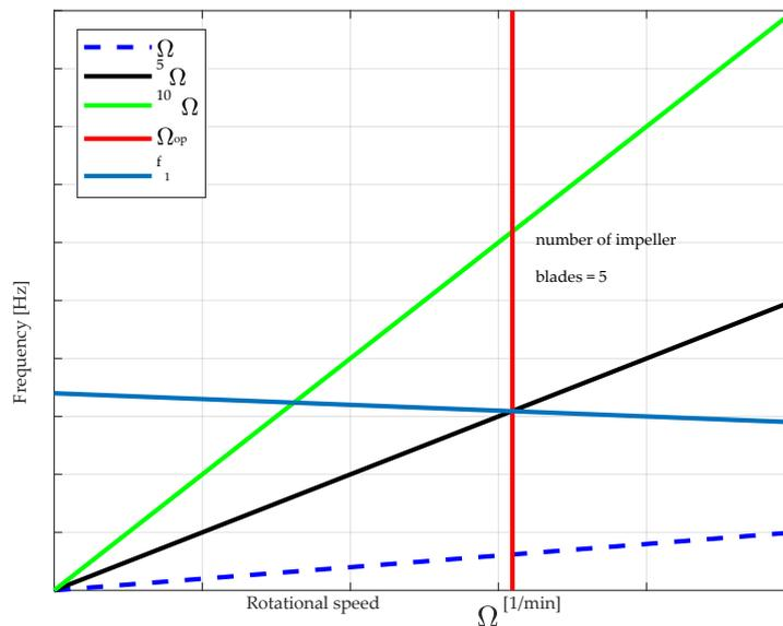
Figure 5 Campbell diagram for the case of a rotor-stator interaction
