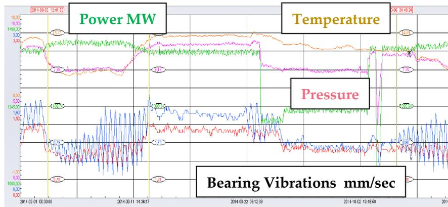
Figure 30 Change of cyclic vibrations due to load-follow of a NPP
