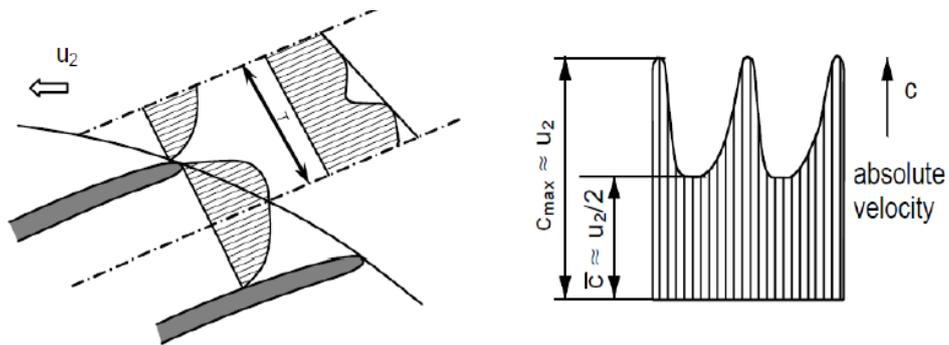
Figure 4 Wake flow in impeller outlet (Gülich, 2010)
