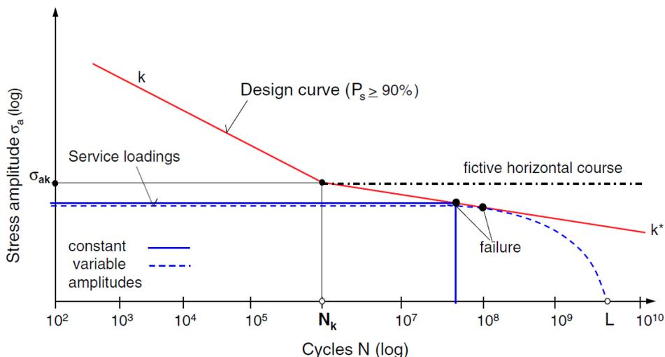
Figure 55 Design against so-called "Fatigue limit"
