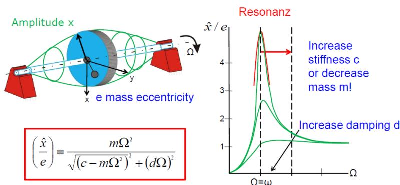
Figure 17 Lateral vibrations of a Laval shaft due to unbalance (Nordmann, 2016)
