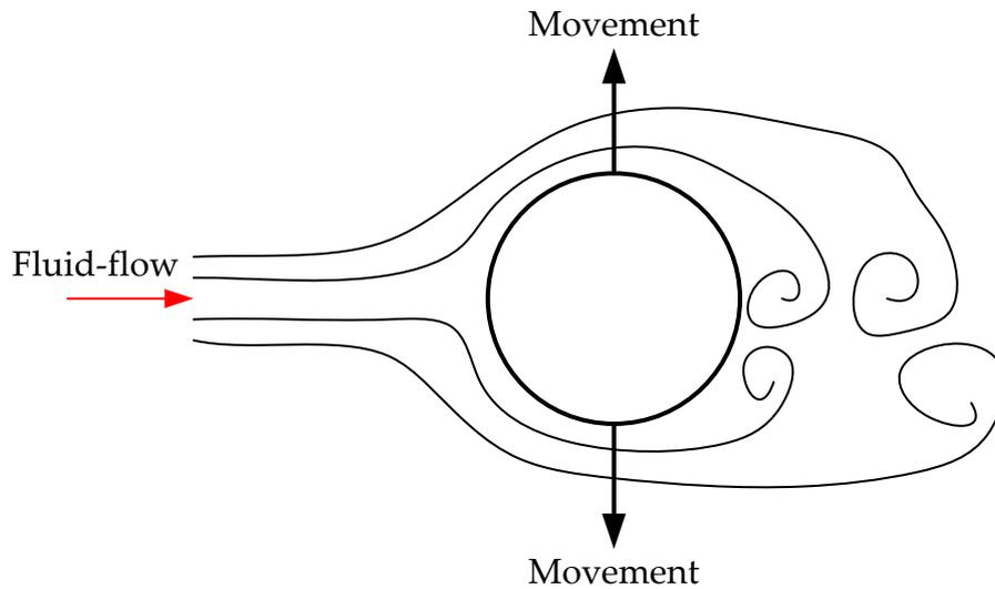
Figure 13 Vortex shedding past a single tube
