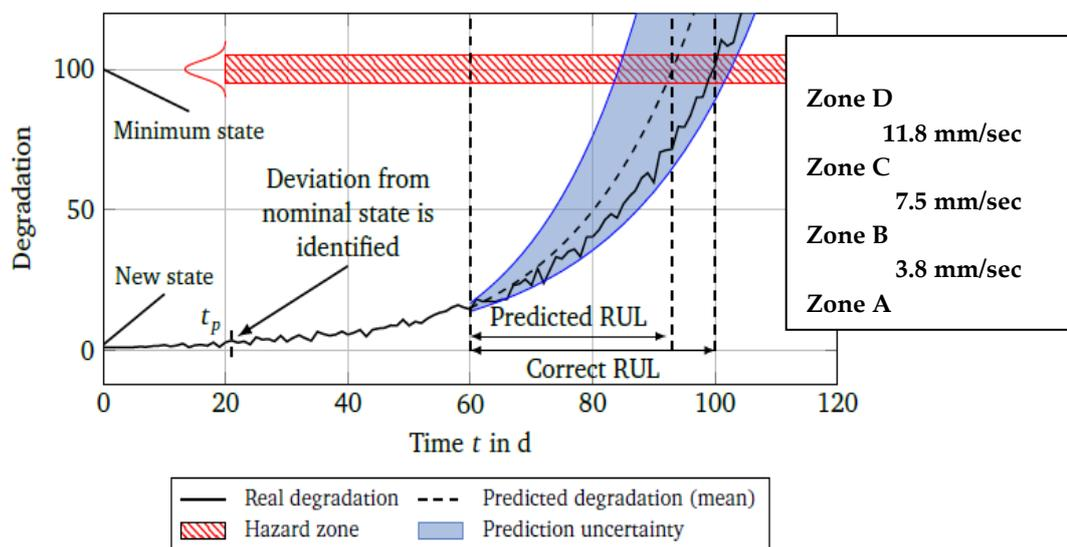
Figure 39 Vibration velocities (degradation) of a component versus time – RUL
