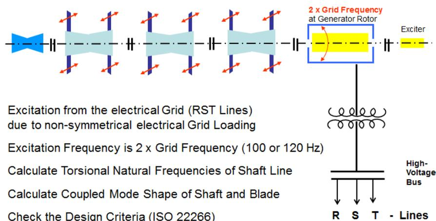
Figure 26 Excitation of the generator shaft line due to non-symmetrical grid loading
