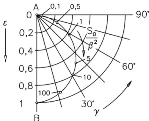
Figure 7 Gümble-curve as the static equilibrium curve for the shaft position (Nordmann, 2016)
