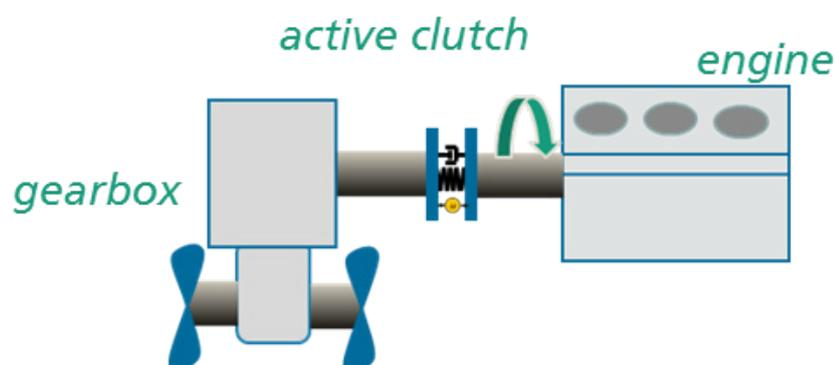
Figure 49 Design for an active clutch in order to reduce torsional vibrations of a drive train
