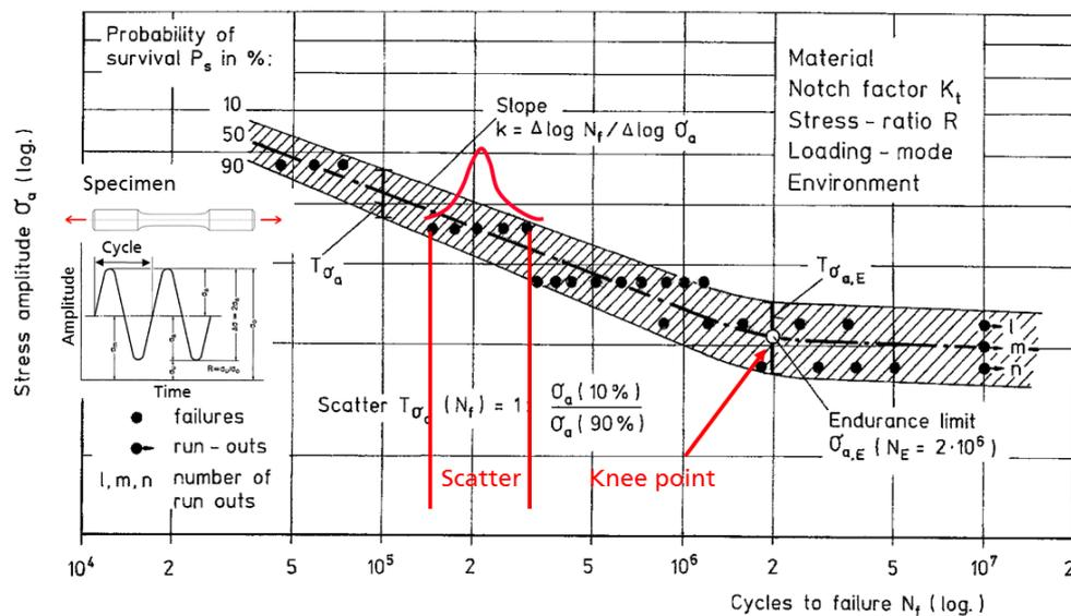
Figure 53 Principle of Woehler-curve (SN Curve)
