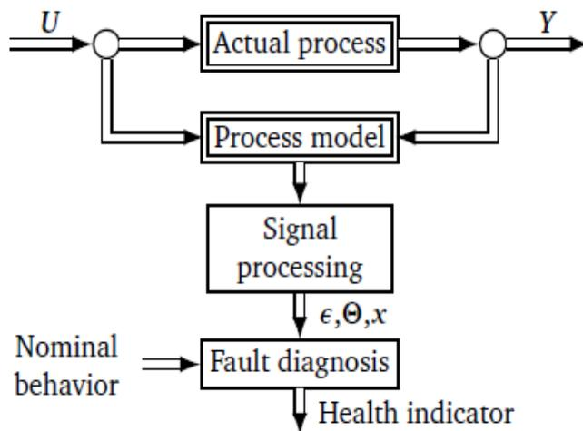
Figure 37 Block diagram of a model-based fault diagnosis
