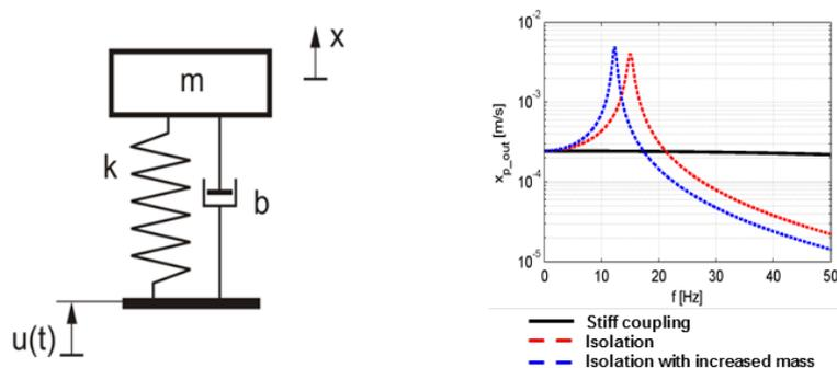
Figure 45 Framework of the system (left figure) and vibration reduction by means of isolating the excitation (right figure)
