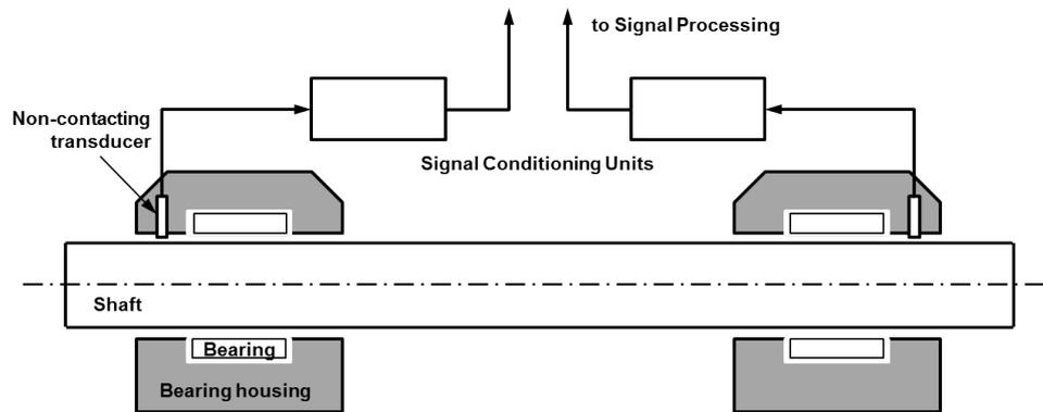
Figure 33 Measuring points for measurements on rotating shafts
