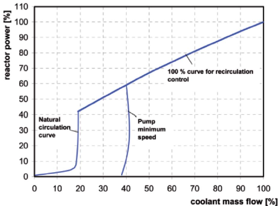
Figure 1 Reactor power of a BWR as a function of the coolant mass flow (Ludwig, et al., 2010)
