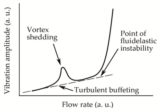
Figure 12 Dependency between vibration amplitude and flow velocities within the heat exchanger (Khalifa, 2011)
