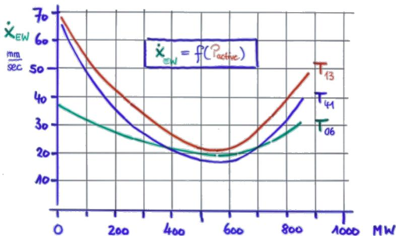
Figure 28 Amplitude of the end-winding vibrations versus the active power of a electrical generator
