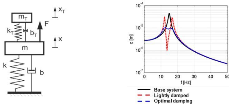
Figure 46 Framework of the system (left figure) and vibration reduction due to compensation (right figure)
