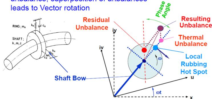
Figure 19 Superposition of a mechanical and thermal unbalance of a shaft (Nordmann, 2016)
