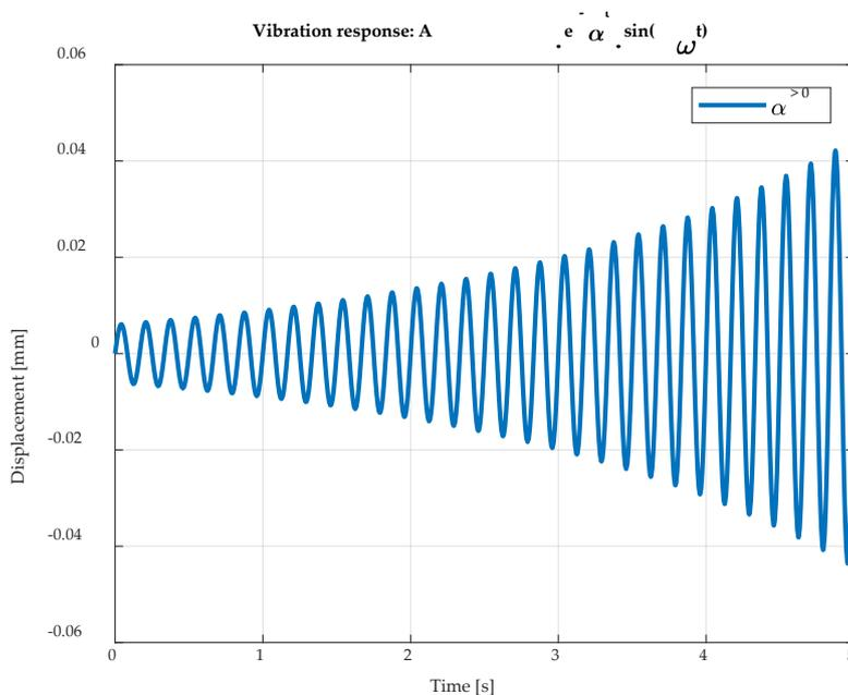
Figure 9 Unstable vibration response of a main recirculation pump
