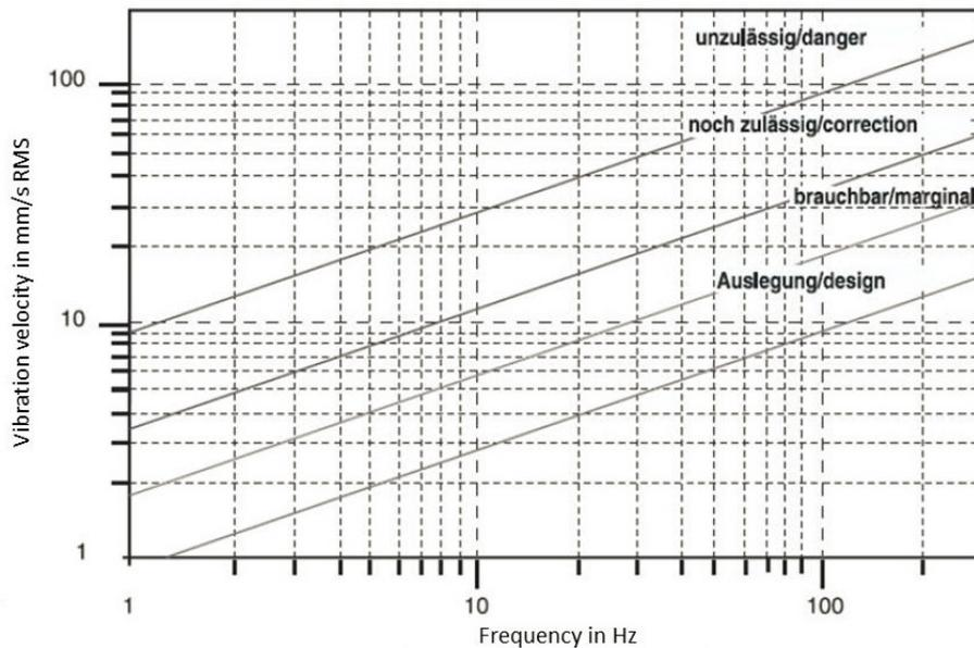
Figure 40 Vibration velocity (rms) limits according to VDI 3842
