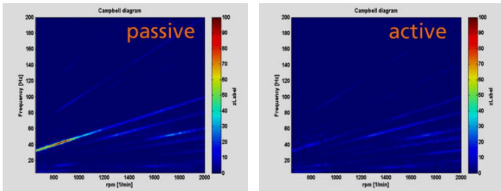
Figure 50 Campbell diagram of the drive train with passive (left) and active clutch system (right)
