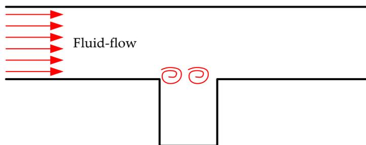
Figure 15 Simplified schematic of a tube with a dead ended side branch and vortex shedding
