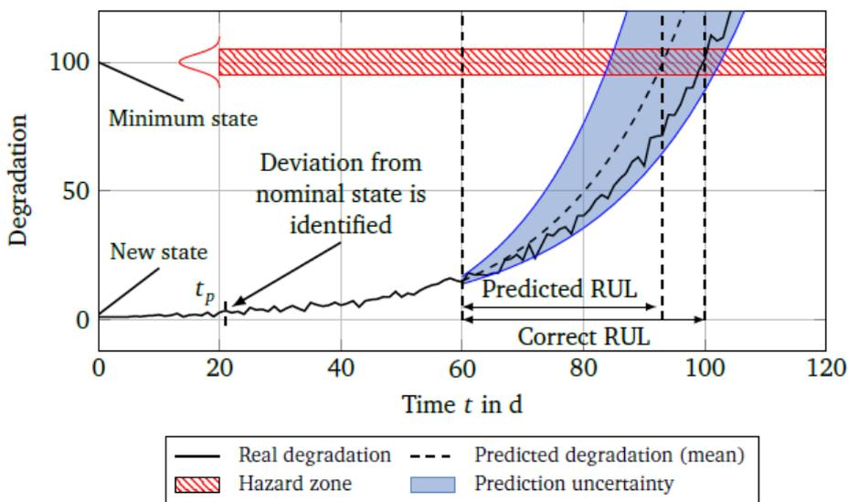
Figure 38 Degradation of a component versus time - remaining use lifetime (Anger, 2017)
