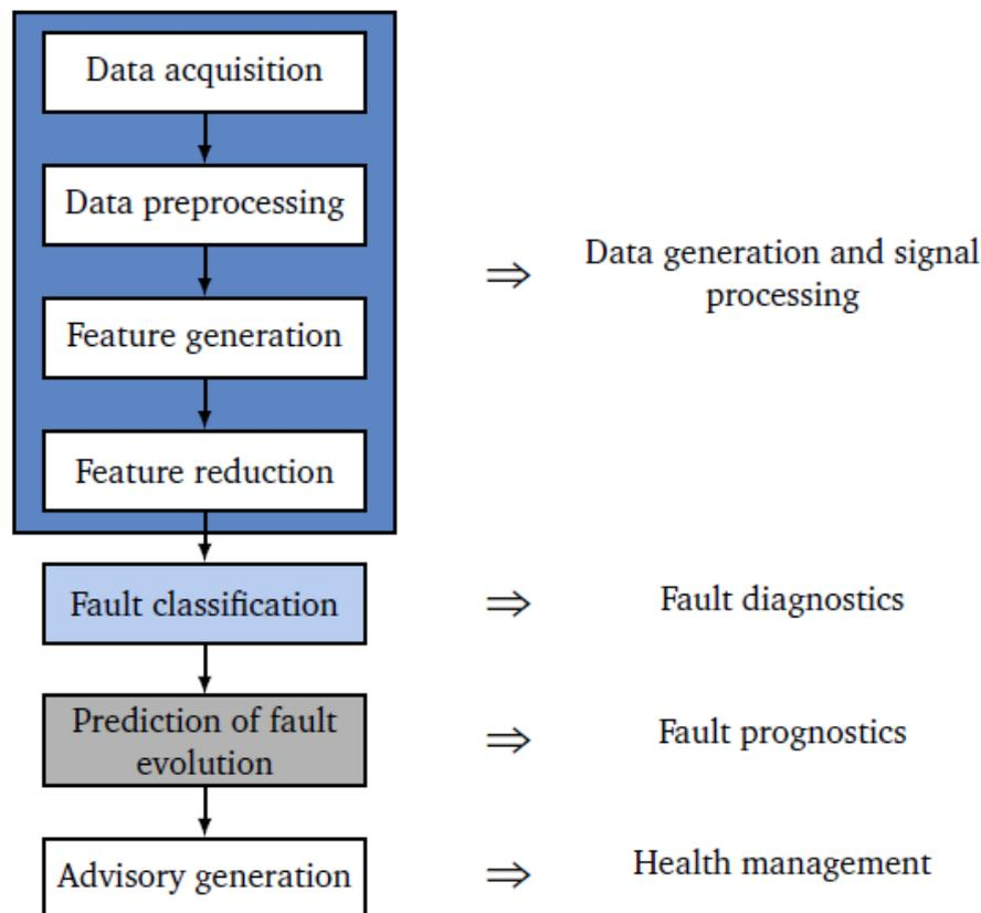
Figure 31 Condition monitoring system including diagnosis, prognosis and health management for NPP components (Anger, 2017)
