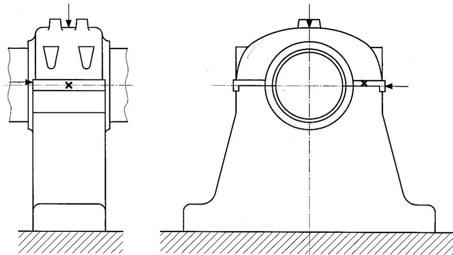
Figure 32 Measurement points for non-rotating parts: bearing pedestal of a turbine
