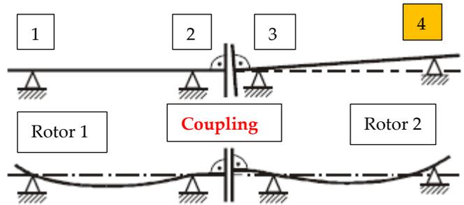
Figure 24 Misalignment in case of two part rotors and four bearings (Nordmann, 2017)
