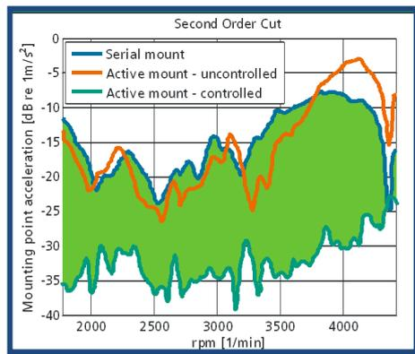
Figure 48 Acceleration-measurement at the active engine mount (second engine order)
