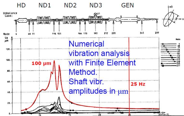
Figure 18 Lateral vibrations of a turbine shaft due to unbalance (Nordmann, 2016)
