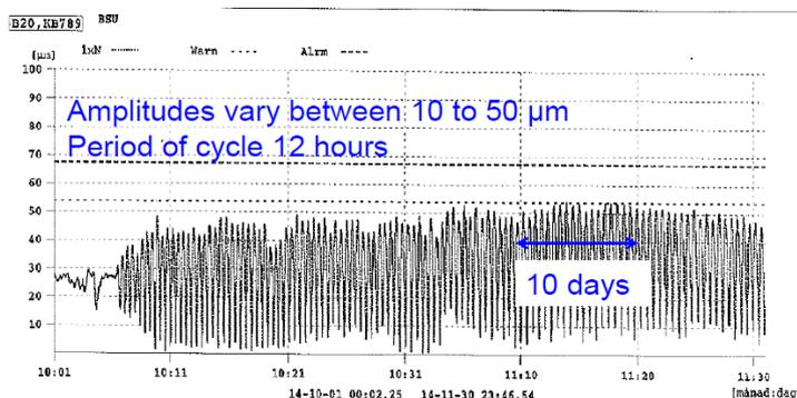
Figure 20 Cyclic vibrations of a turbine shaft train (Nordmann, 2016)
