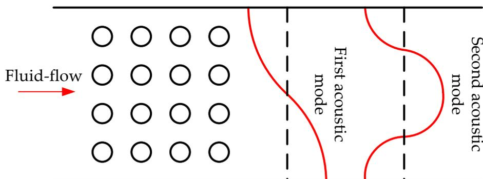
Figure 14 Simplified schematic of a tube bank in a heat exchanger with the associated first and second acoustic modes (Ziada, 2006; Fiorentin, et al., 2017)
