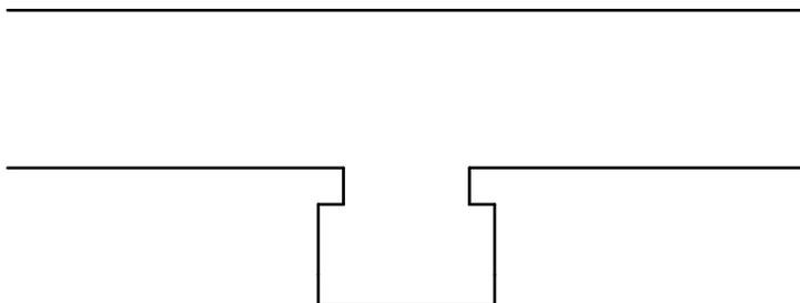
Figure 16 Fluid-flow and vortex shedding in a pipe with a dead ended side branch (Helmholtz resonator)
