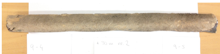
Figure 26. Material 4 (left part of tube) and material 5 (right part of tube) after exposure in the superheater (SH-HT). Removed from site in 2017.
