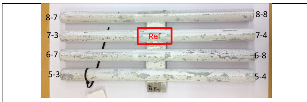
Figure 65. Photographs of the samples after exposure at Ørsted /Avedøre in the superheater (SH-1-LT). The tubes were removed from the site in 2017. A reference sample (indicated) was taken from the middle non-coated region.
