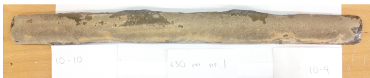
Figure 27. Material 10 (left part of tube) and material 9 (right part of tube) after exposure in the superheater (SH-HT). Removed from site in 2017.
