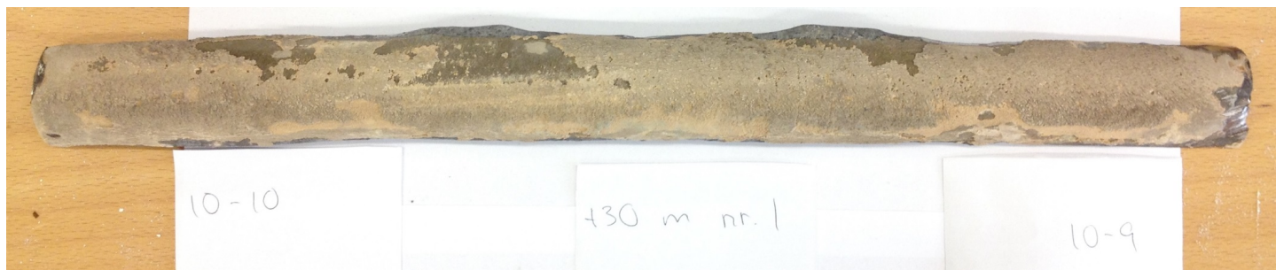
Figure 92. Material 10 (left part of tube) and material 9 (right part of tube) after exposure in the superheater (SH-HT). Removed from site in 2017.
