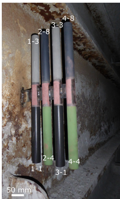
Figure 68. Photograph of the samples mounted in position C in Avedøre before exposure. Sample ID indicated in the image. The scale bar is approximate.
