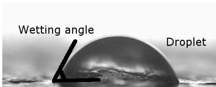
Figure 4. Typical droplet on material 1 after wear test 10 h, before water wash.
