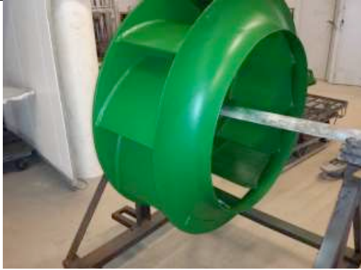
Figure 56. The flue gas fan after application of CMP in 2013
