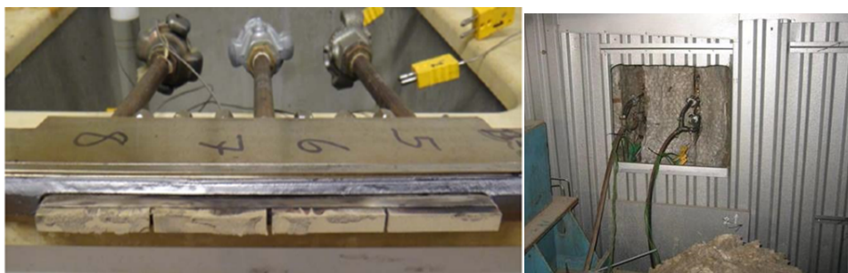
Figure 4. Vattenfall's wall probe after exposure (left). The probes sit vertically in a slit in the fin between two tubes, here seen from outside the furnace, (right).
