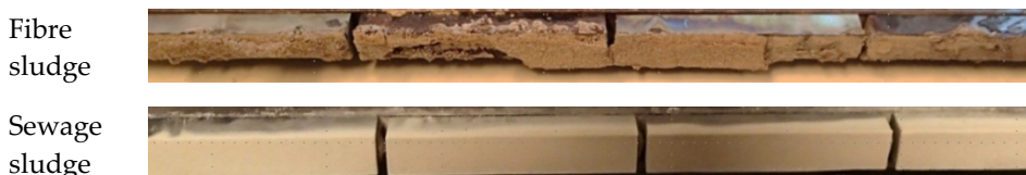
Figure 25. Visual appearance of the sample surfaces after exposure when firing waste wood fuel and fibre sludge (upper) sewage sludge (lower).
