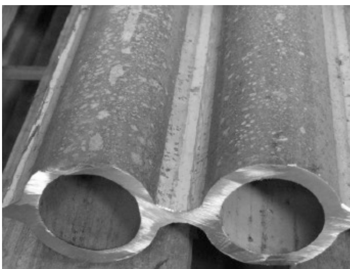
Figure 1. Photograph of part of a furnace wall before being installed in a boiler.
