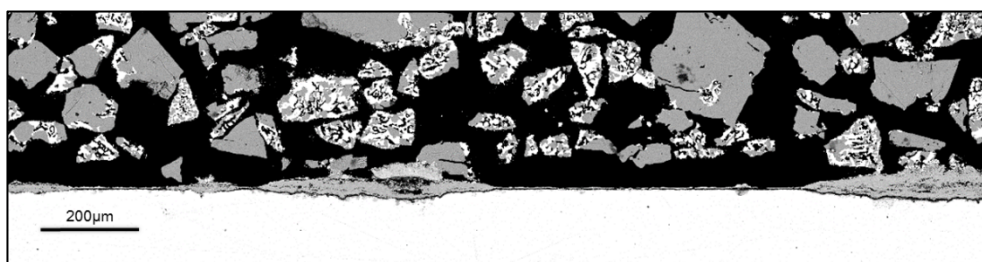
Figure 23: Panorama image of P235GH after exposure to KCl-PbCl 2 -ZnCl 2 without SO 2 at 350 °C.
