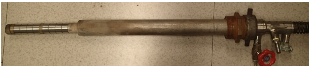
Figure 2. Probe used in the 8h gradient probe tests.
