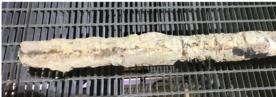
Figure 13. Probe exposed 1000h in the Sulfur Recirculation line (first) and 1000h in the reference line (after)
