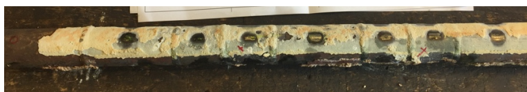
Figure 16. Superheater after 6 months in Sulfur Recirculation line
