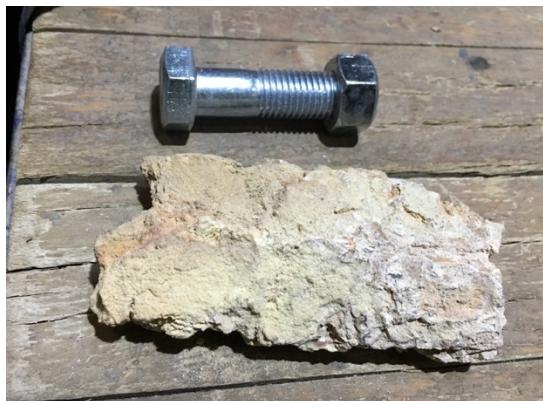
Figure 17. Piece of deposit extracted from the Sulfur Recirculation line after 2000h exposure
