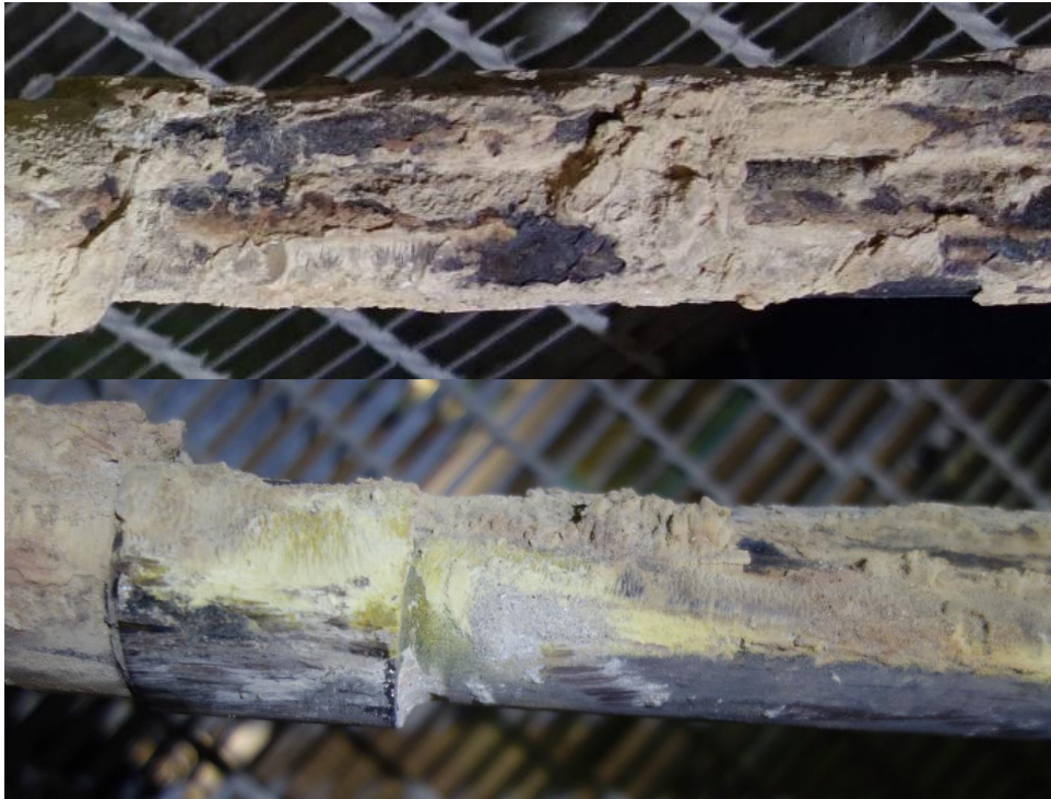
Figure 12. Photographs of the corrosion probes after 1000 + 1000 h Ref (top) and 1000 + 1000 h Rec (lower).
