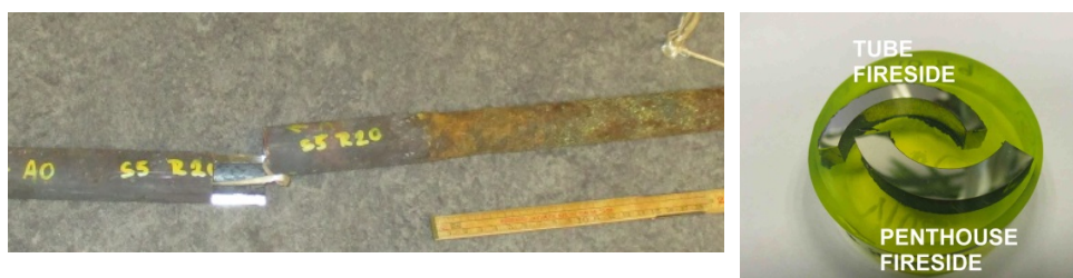
Figure 11: Tube examined for TP347H FG where section consists of both penthouse exposure and boiler exposure
