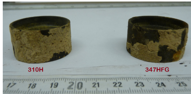
Figure 118 Exposed weight loss samples before cleaning.
