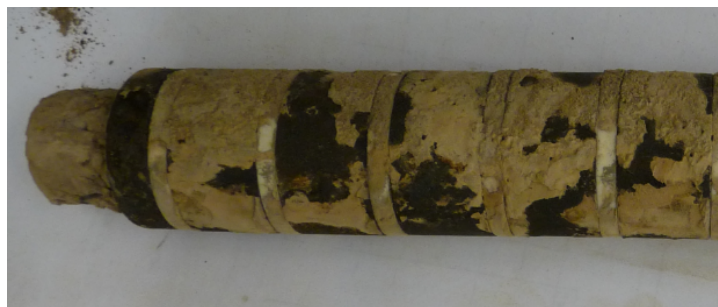
Figure 117 Online corrosion probe after the test campaign 1.
