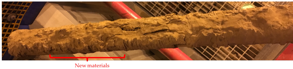
Figure 101. Probe with the samples (a) before and (b) after 144 hours with ammonium sulphate addition
