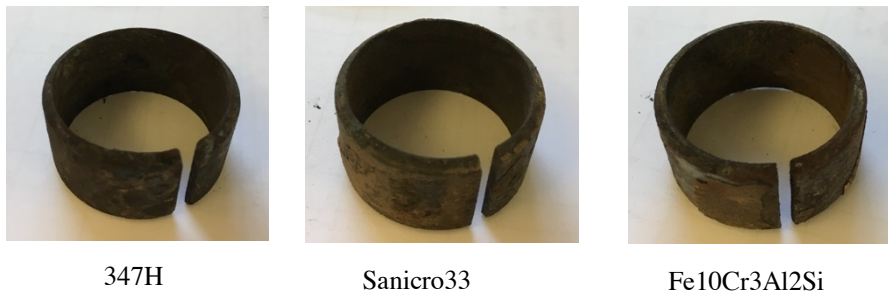
Figure 94. Optical image of the samples after 144 hours exposure with ammonium sulphate addition
