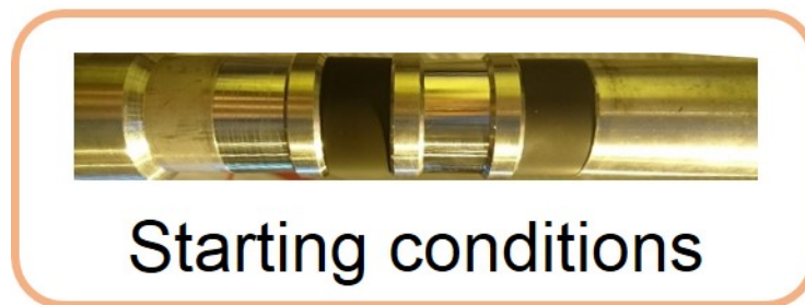
Figure 40. Initial conditions of the ring samples prior exposure; clean / pre-oxidized / clean / pre-oxidized.
