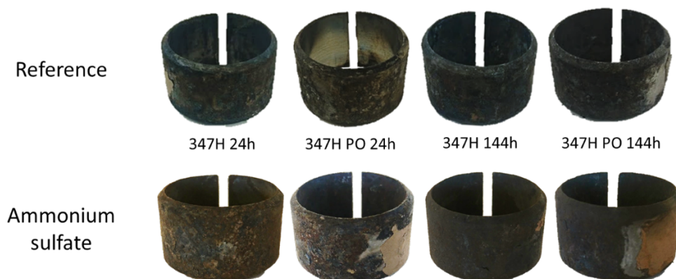
Figure 53. Optical images of exposed samples after 24 hours and 144 hours with and without ammonium sulphate
