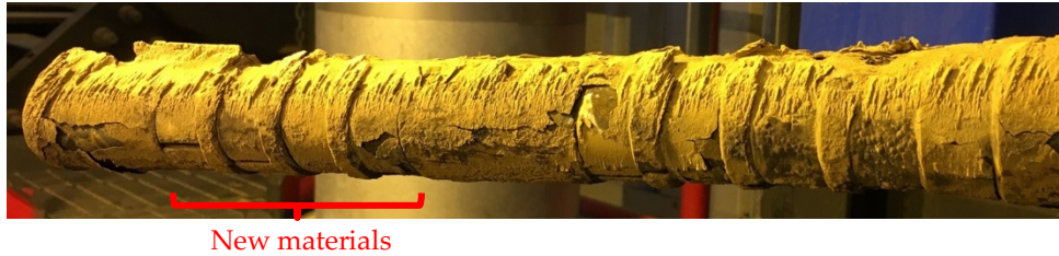
Figure 93. Probe with the samples (a) before and (b) after 144 hours exposure with ammonium sulphate addition
