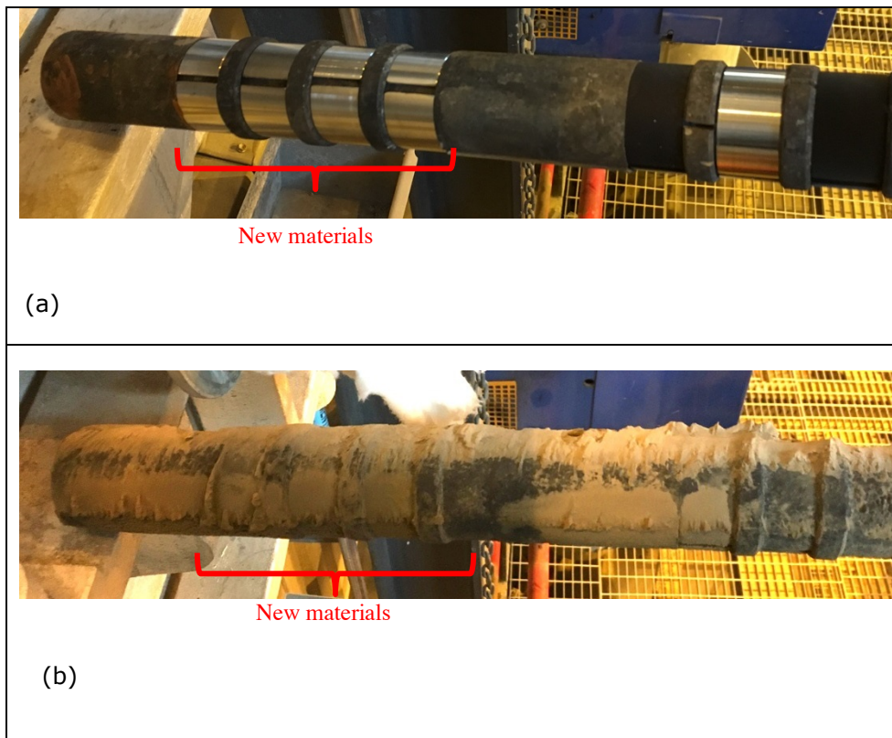
Figure 71 (a) Probe with the samples before exposure (b) Probe with the samples after 24 hours exposure in regular fuel conditions
