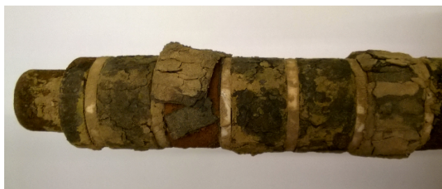
Figure 123. Online corrosion probe after the test campaign 3.
