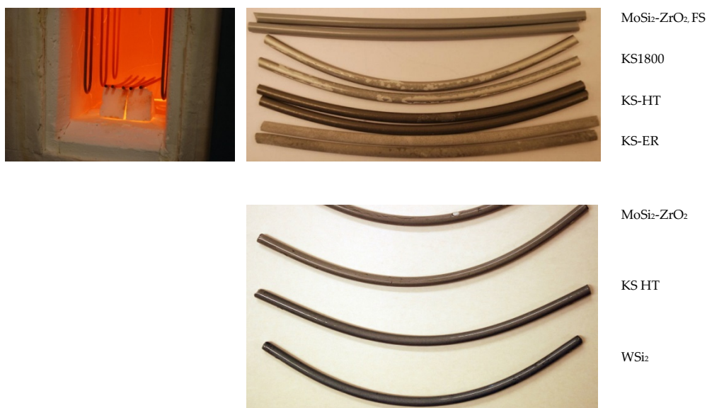
Fig. 5 Sag tests in air at 1600 and 1700°C for 100 h; the sag testing setup (left), testing bars of different materials after sagging at 1600°C (upper right); testing bars sagged at 1700°C.
