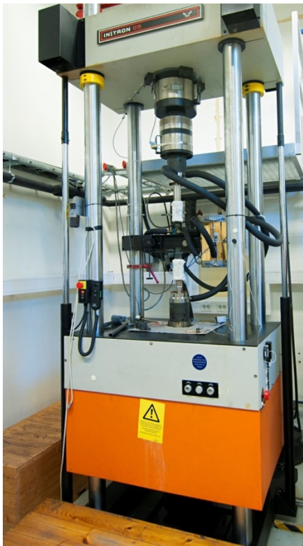
Figure 33. LCF machine for component testing.
