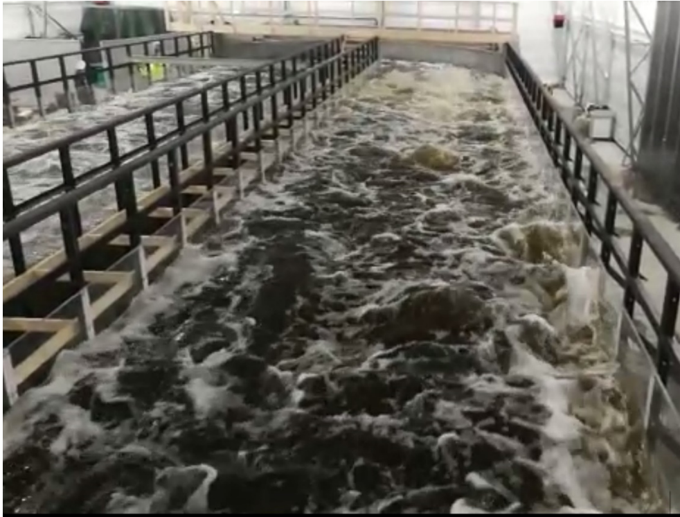
Figure 6 The new test facility, a flume at Vattenfall Laboratory. Photo: David Aldvén
