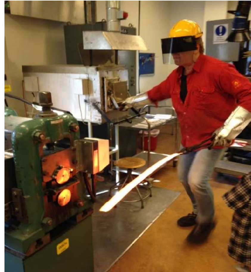
Lab scale vacuum melting and hot rolling
