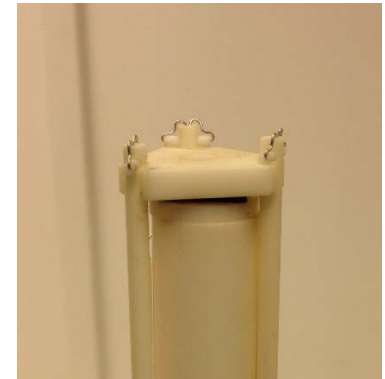
Sample mounted on Probostat, inclusive Pt-electrode
