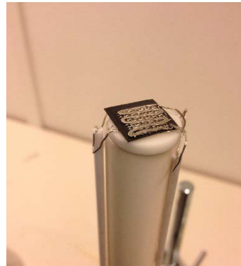
Sample mounted on Probostat, inclusive Pt-electrode
