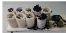
Alloy specimens after metal dusting test at 620 °C.
