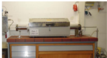
Exposure setup of high pressure tests
