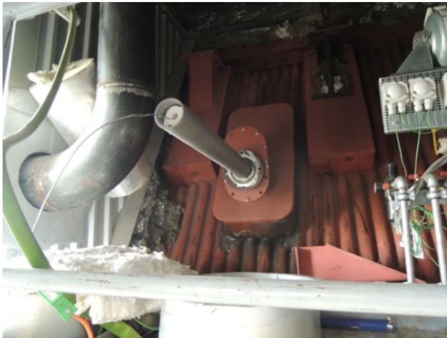
Pre-oxidized FeCrAl tube exposed at the steamboost position at 900 C
