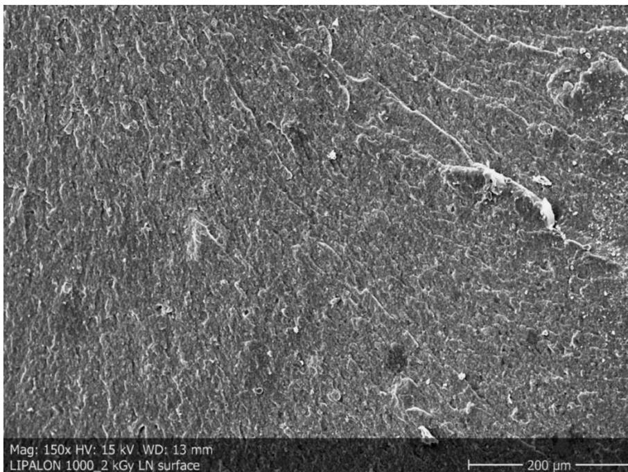
Figure 14. Fracture surface of Lipalon sample after irradiation of 1 MGy absorbed dose.
