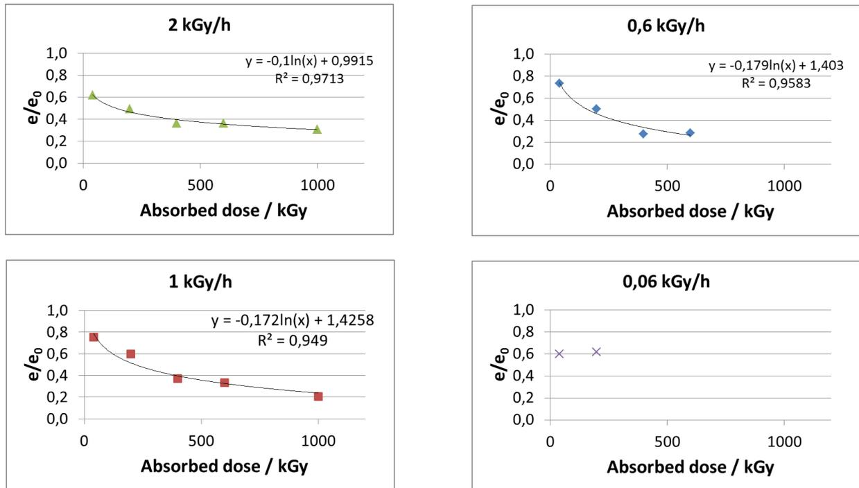
Figure 11. Extraction of end-point criteria from experimental data.
