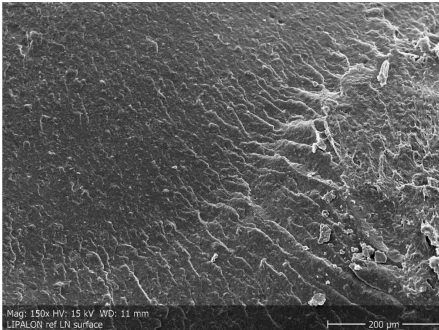
Figure 13. Fracture surface of Lipalon reference sample.
