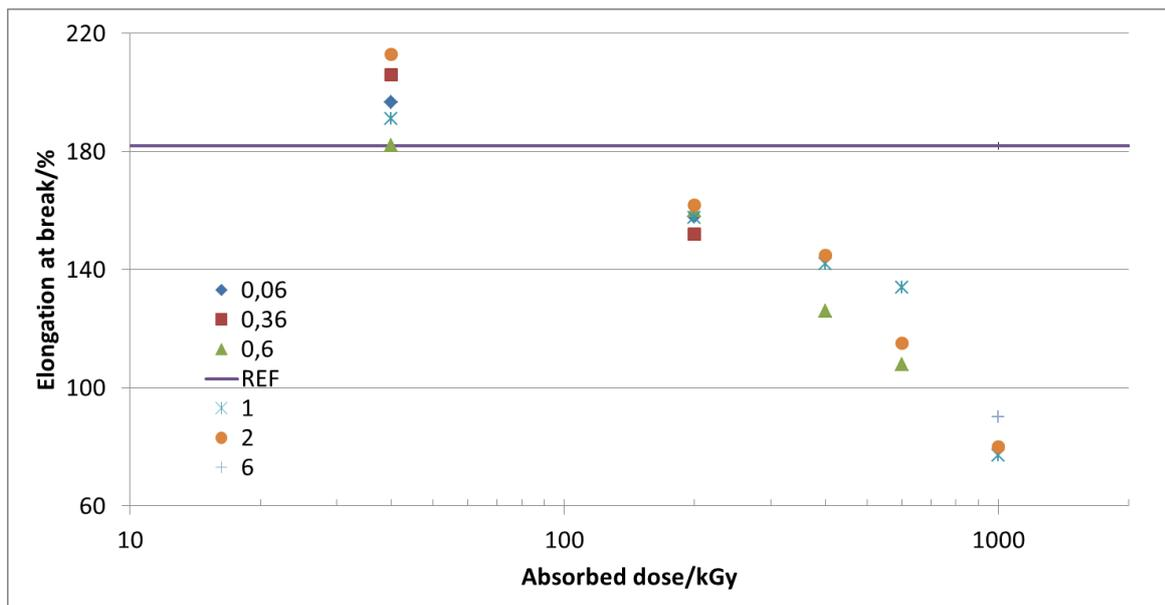
Figure 3. Elongation of break of EPDM at different dose rates as function of absorbed dose.
