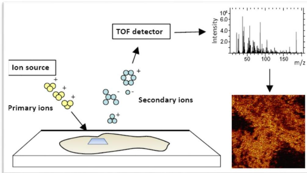
Figure 2. Illustration of the ToF-SIMS technique.
