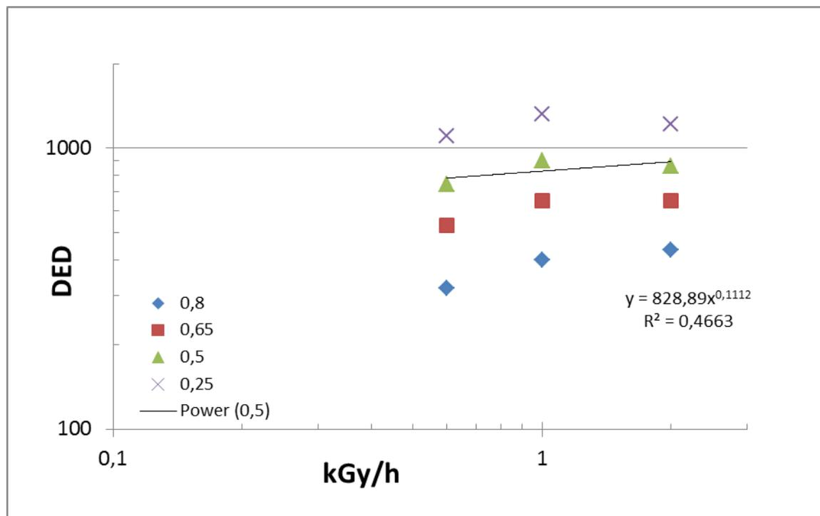
Figure 6. Extrapolation of end-point dose to lower dose rates for EPDM.
