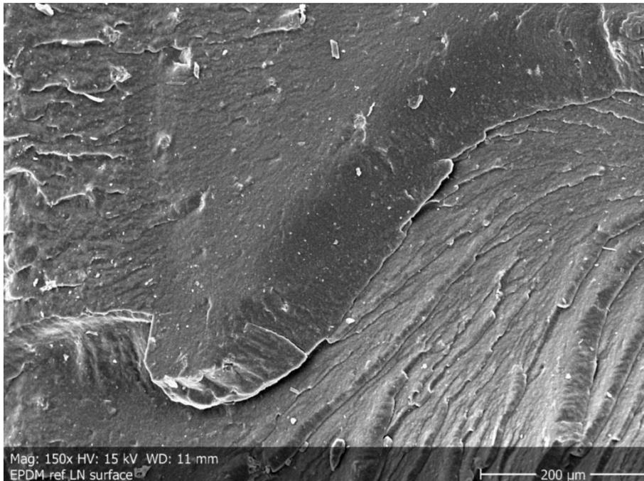
Figure 7. Fracture surface of EPDM reference sample.
