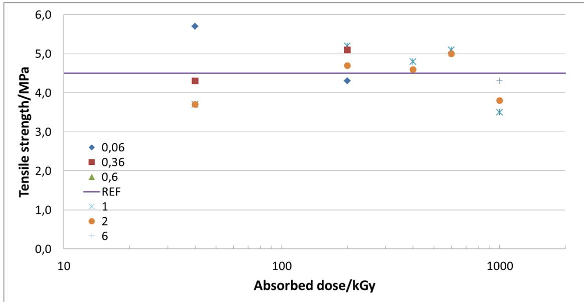
Figure 10. Tensile strength of Lipalon at different dose rates as function of absorbed dose.
