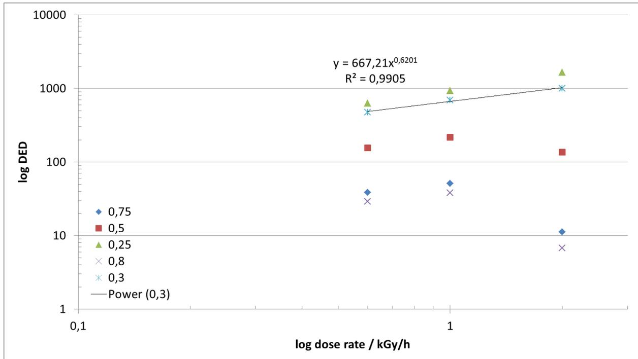
Figure 12. Extrapolation of end-point dose to lower dose rates for Lipalon.
