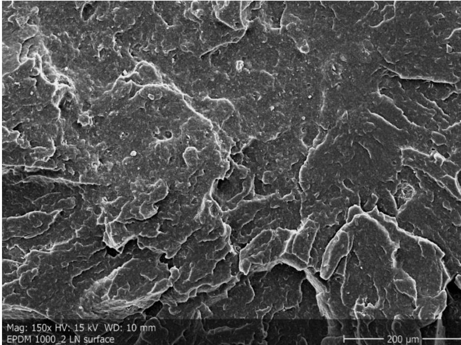
Figure 8. Fracture surface of EPDM sample after irradiation of 1 MGy absorbed dose.
