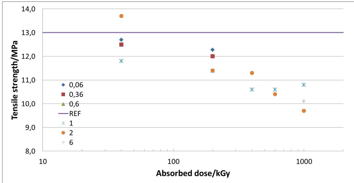
Figure 4. Tensile strength of EPDM at different dose rates as function of absorbed dose.
