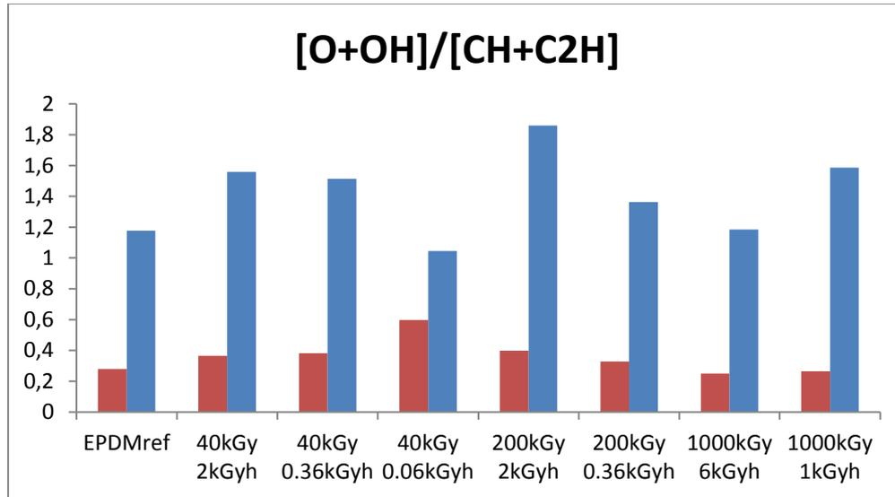
Figure 15. The red bars show total oxygen content in the bulk material and the blue bars the surface material. The surface seems to contain higher concentration of oxygen containing reaction groups.
