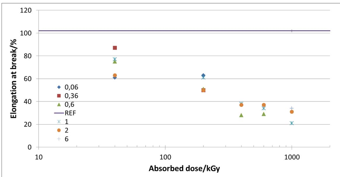
Figure 9. Elongation of break of Lipalon at different dose rates as function of absorbed dose.
