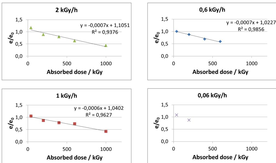
Figure 5. Extraction of end-point criteria from experimental data.
