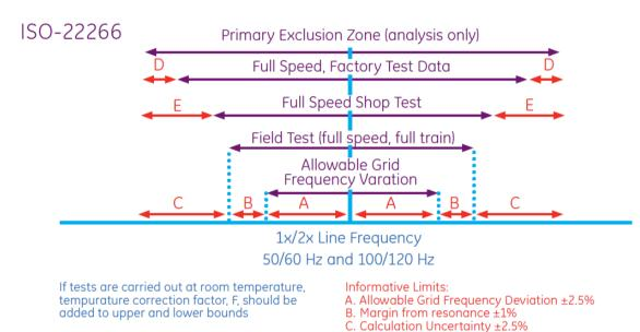
D. Full-speed generator, static LP test ±1% E. Full-speed generator and LP test ±2%
