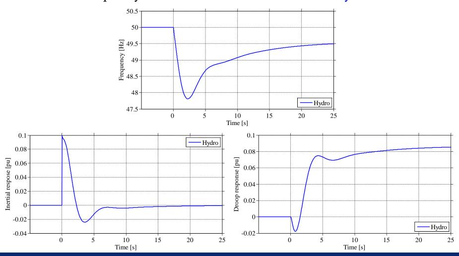
2. How does the power system inertia affect the frequency stability?
