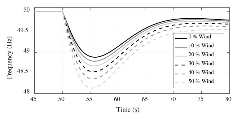
A reduced system inertia  $(H_{sys})$  cause lower frequency nadirs and steeper frequency derivatives during disturbances.
