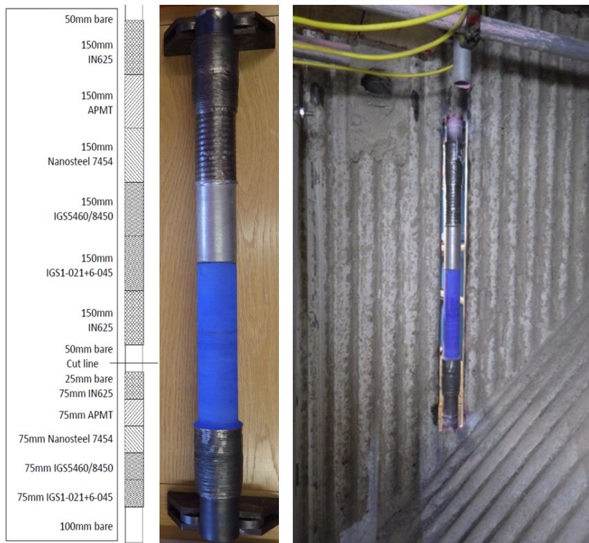
Fig. 2.2.7. Sketch of coated tube showing dummy tube at bottom and furnace wall tube at top (left). Photograph of the wall tube before being welded into position (middle). Photograph of the tube in position in furnace wall (right).
