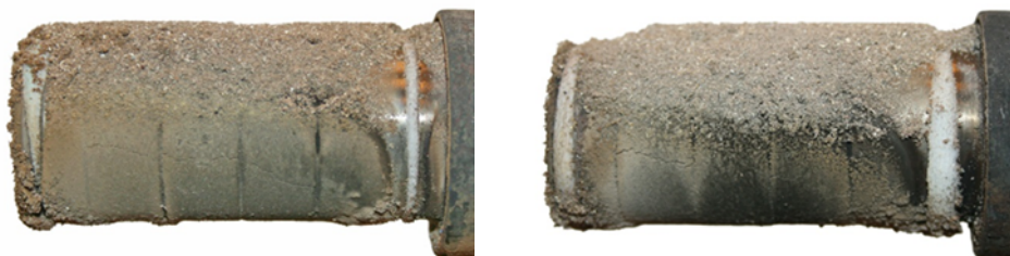
Fig. 3.2.1 Furnace wall probe at 380°C directly after removal from the test rig. Fuel 1 (left); Fuel 2 (right)
