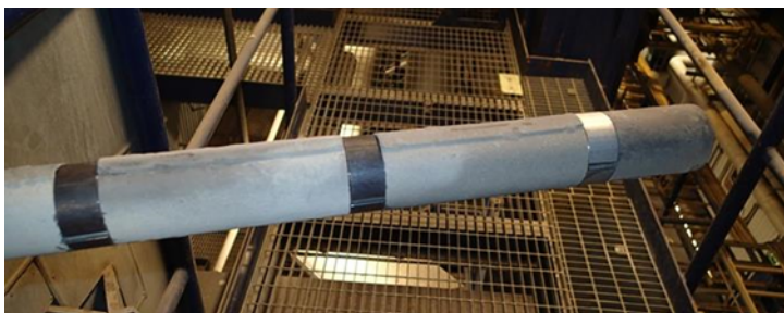
Fig. 2.2.2. Vattenfall's deposit probe before exposure.
