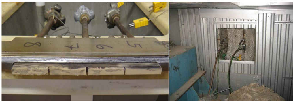
Fig. 2.2. 1. Vattenfall's wall probe after exposure (left). The probes sit vertically in a slit in the fin between two tubes, here seen from outside the furnace, (right)
