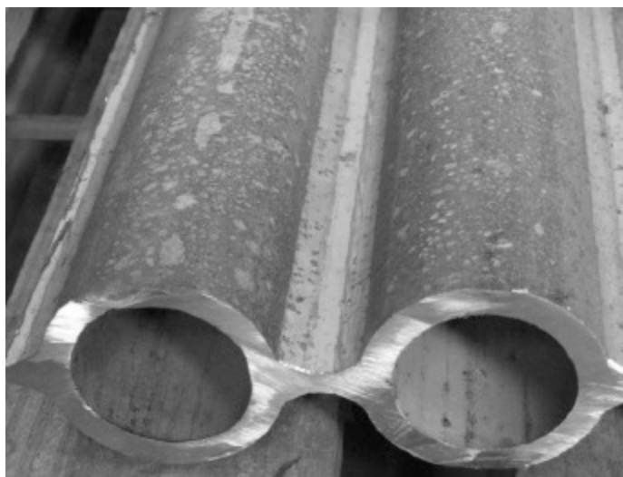
Fig 1.2.1. Photograph of part of a furnace wall before being installed in a boiler.
