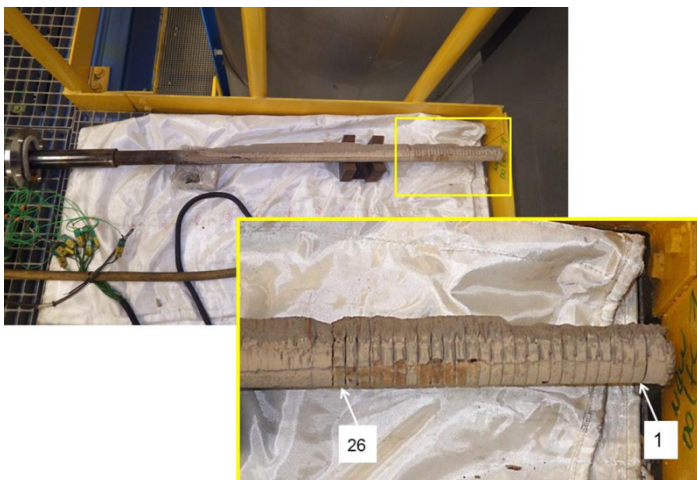
Fig. 2.2.5 . E.ON's superheater probe after 890 hours exposure (close up of probe tip with ring specimens).
