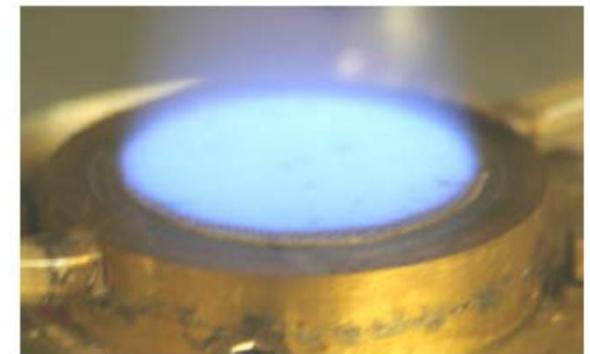
1D flame stabilized on the heat flux burner.
