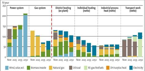
Electrification and integration between energy sectors helps integrating large amounts of wind power (>50 %) Source: Energinet.dk. 2015. Energy Concept 2030 – Summary. An analysis of concepts and development paths to sustain a competitive and strong RE based energy system. 16
