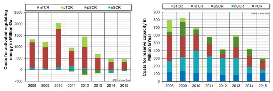
PCR Primary, SCR Secondary and TCR Tertiary control, p for positive and n for negative. Costs for activated energy (left) and reserved capacity (right) Source Hirth, L., Ziegenhagen, I. Balancing Power and Variable Renewables: Three Links. <sub>5/2017</sub>Renewable & Sustainable Energy Reviews.
