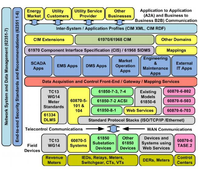
e.g. The IEC 60870 is a set of standards which define systems used for tele-control in supervisory control and data acquisition (SCADA) in electrical engineering and power system automation applications.
