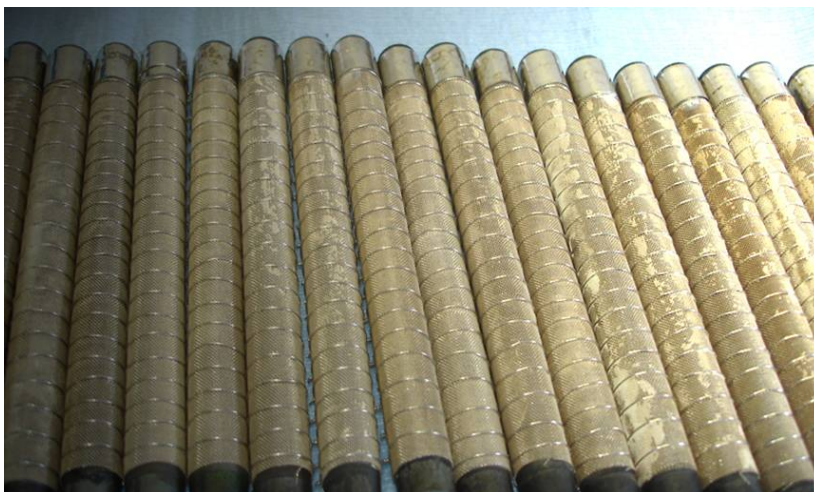
Figure 11. MSRI tubular anode supported SOFC design [www.msrihome.com].
