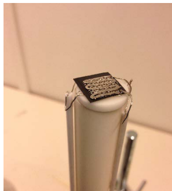
Sample mounted on Probostat, inclusive Pt-electrode
