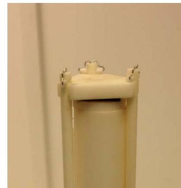
Sample mounted on Probostat, inclusive Pt-electrode
