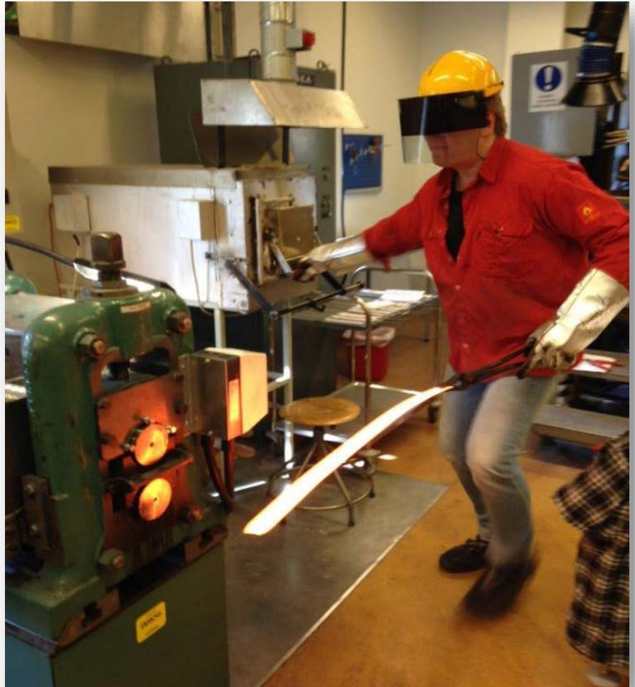
Lab scale vacuum melting and hot rolling
