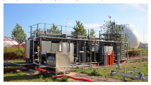
Figure 11 Cryogenic biogas upgrading and liquefaction, pilot plant from Cryo Pur, Valeton, France
