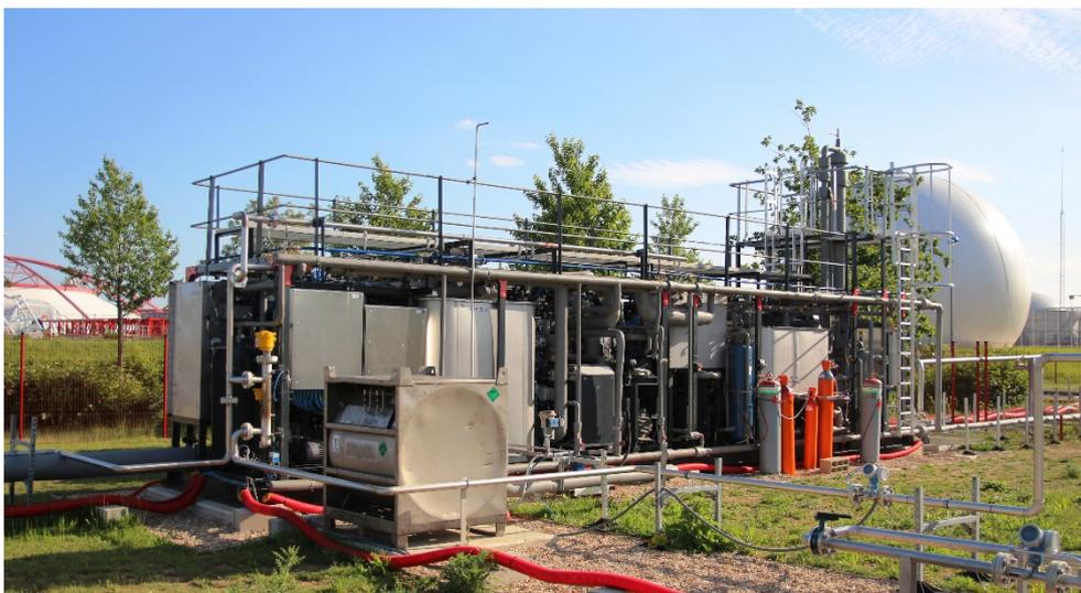
**Figure 11 Cryogenic biogas upgrading and liquefaction, pilot plant from Cryo Pur, Valetton, France**
