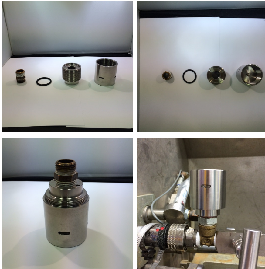
Figure 1. The above pictures shows the test block taken apart (a,b) and mounted together (c). The last picture (d) shows the test block when in place at the tightness test. The material is Stainless steel 316L.
