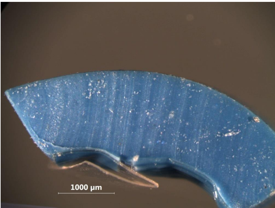
Figure 4: Cross section of unaged Lipalon tensile specimen.
