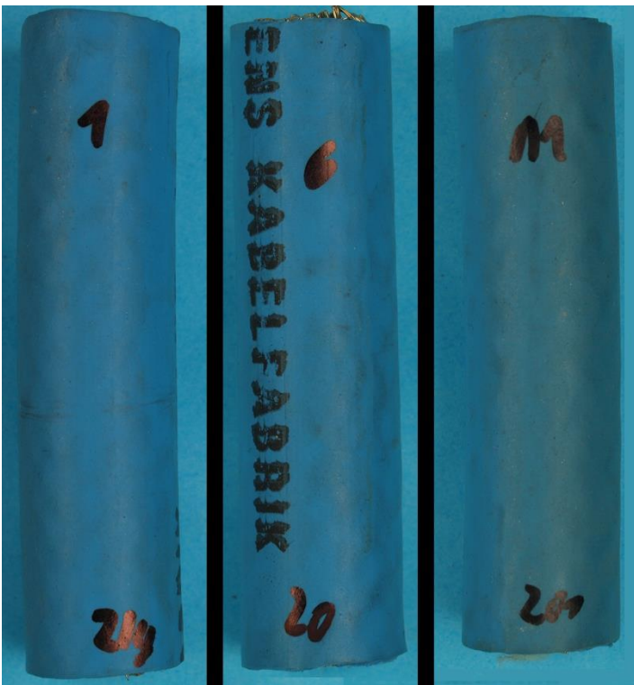
Figure 2: Lipalon cables after irradiation ageing at 28,6°C. From left to right: total absorbed dose 2,3 kGy, 23,3 kGy and 228 kGy, respectively. The used dose rate during all irradiations was 0,39 kGy/h
