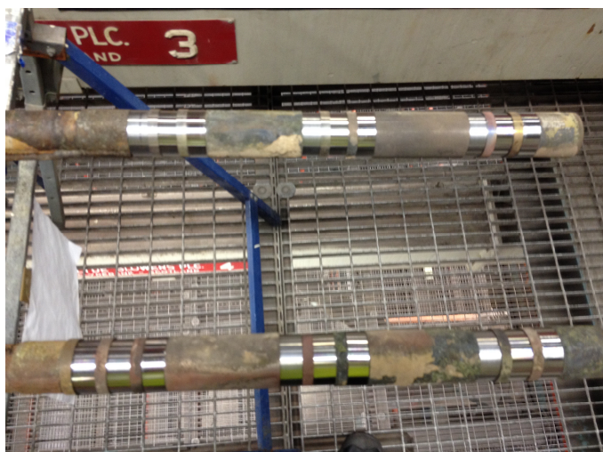
Figure 6. Detail of the samples placed in the probes and temperature zones
