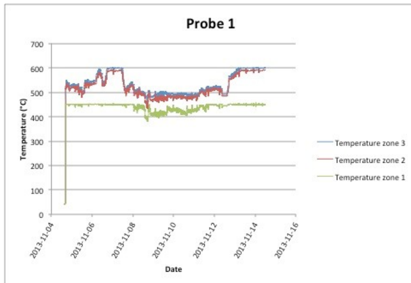
Figure 12. Evolution of the temperature in the P13 boiler during the step 2
