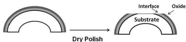
Figure 3. Schematic drawings of tube samples before and after polishing
