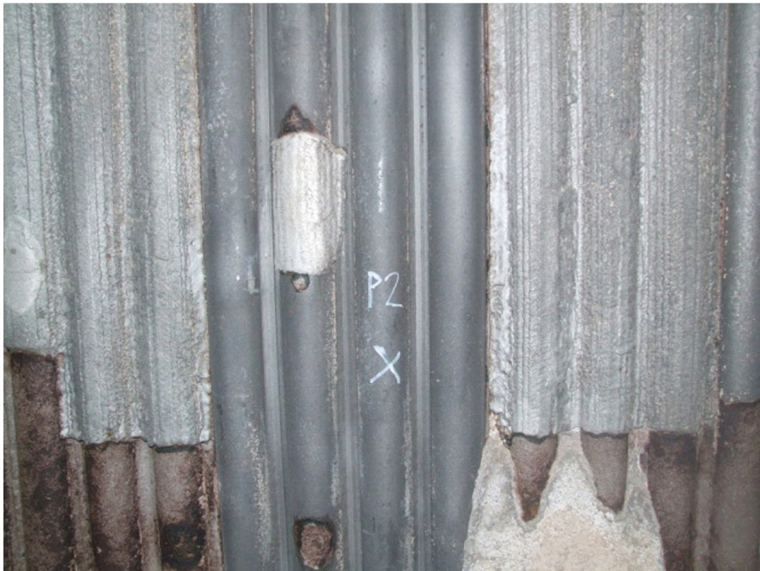
Figure 6 Sample P2: Sumeboil 70C (625 + C) HVOF. The coating was applied in summer 2008 on tubes 45-48.. The sample was taken from tube number 47.
