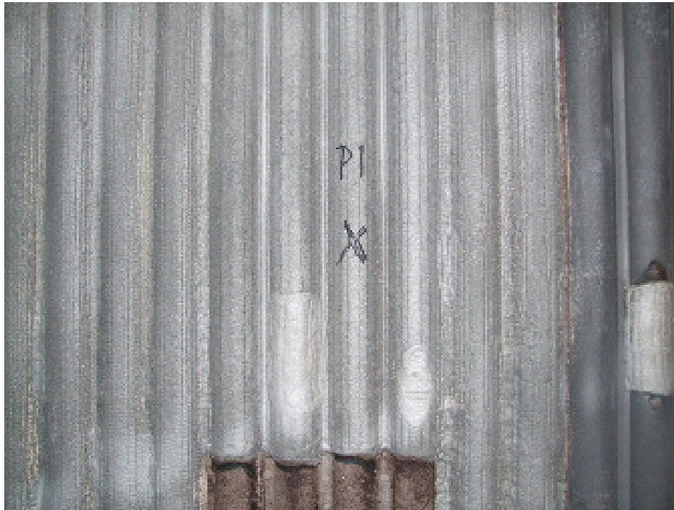
Figure 5 Sample P1: IN625 Arc welded. The coating was applied during summer 2008 by Burmeister and Wain Energy. The sample was taken from tube number 41.
