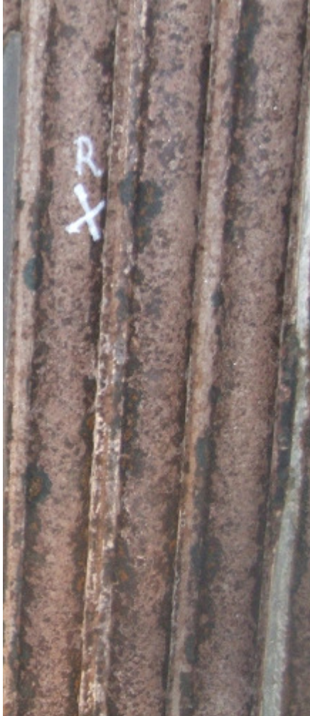
Figure 8 Sample Ref: Un-coated sample from 2011, base material 16Mo3. The sample was taken from tube number 61.
