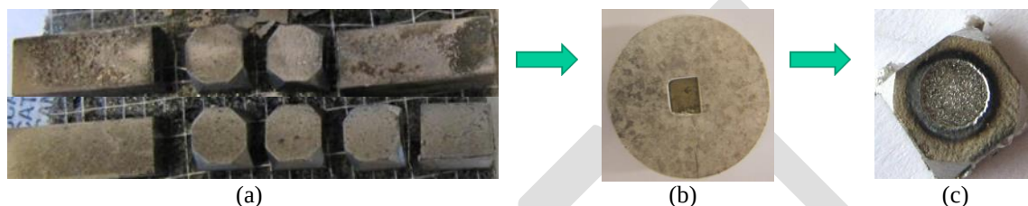
Figure 3. Sample preparation prior to GD-OES analysis (a, b) and sample after GD-OES analysis (c).
