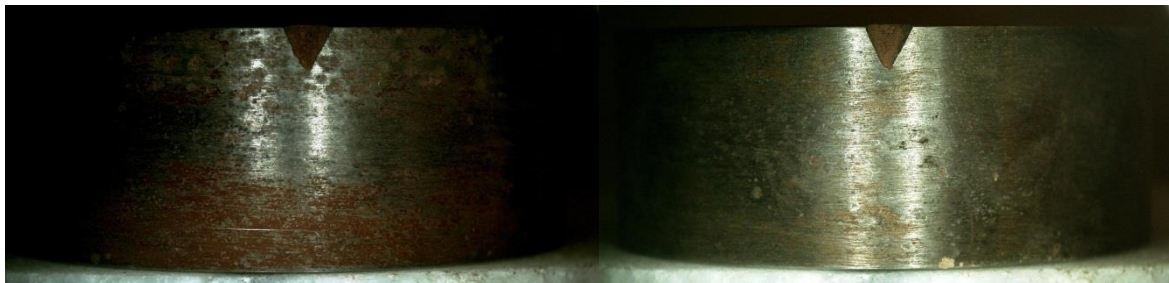
Figure 76. Photos of 253 MA-steel rings from the BW position, leeward side, after deposit removal. Left) PbO. Right) PbO+SWS.
