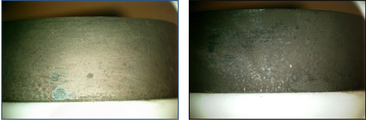
Figure 45. Photos of the windward sides of the 16Mo3 rings after deposit removal (BW position). Left) Ref 2, Right) SWS2.
