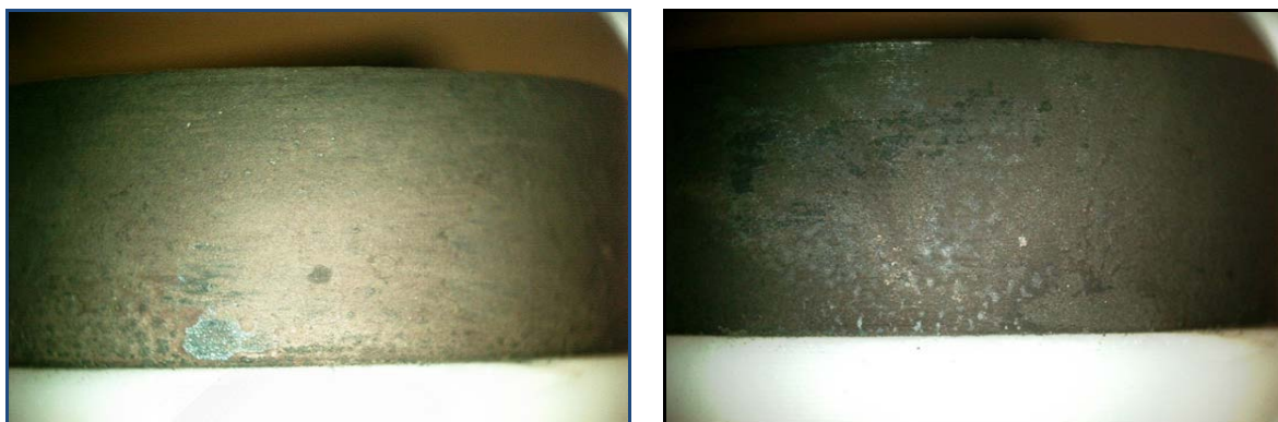
Figure 61 Photos of the windward sides of the 16Mo3 rings after deposit removal (BW position). Left) Ref 2, Right) SWS2.
