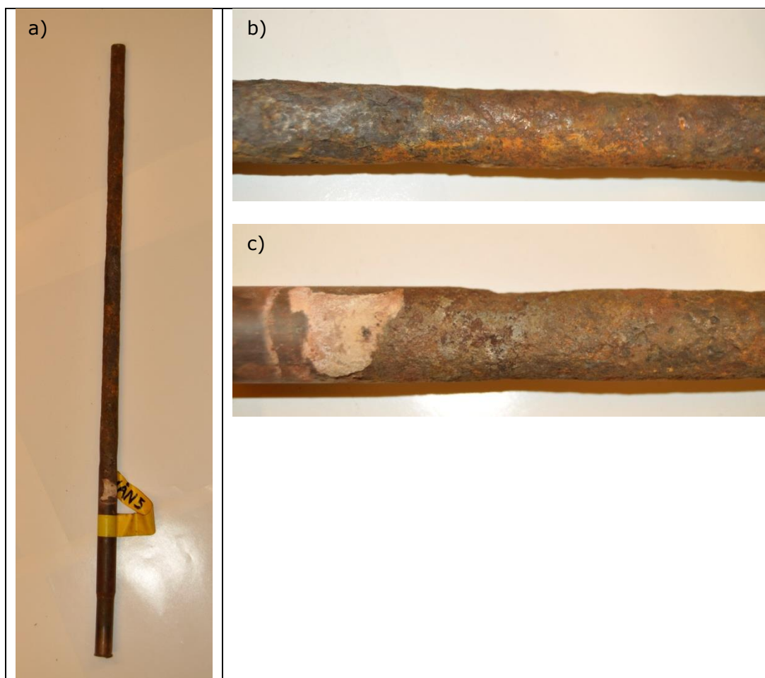
Figure 6-58. Images of the thermal shield tube exposed at position KT043.
