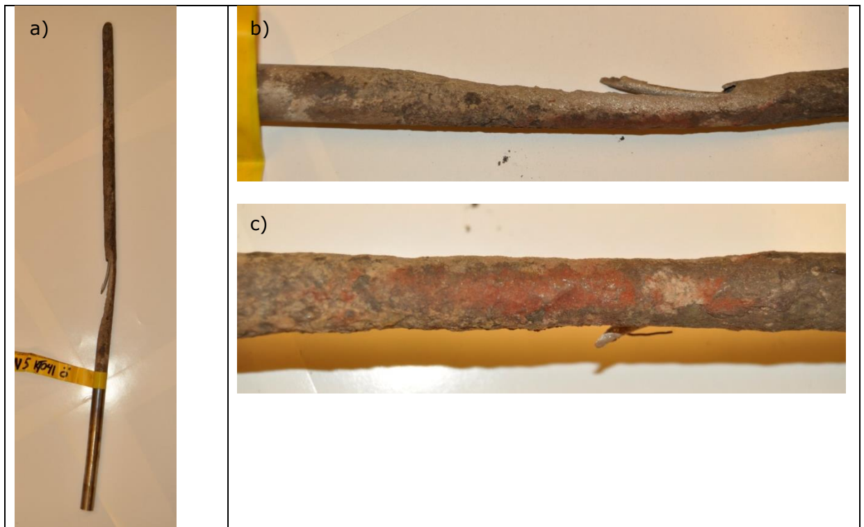
Figure 6-66. Images of the thermal shield tube exposed at position KT041:Ö.
