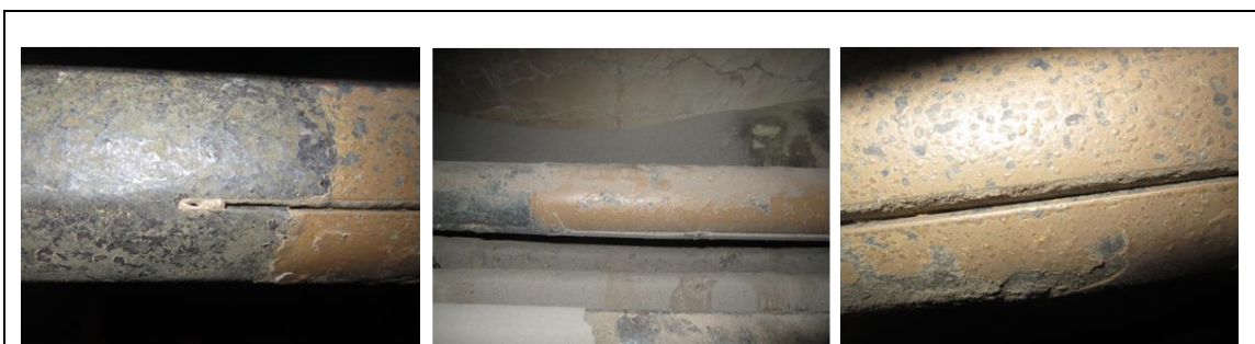
Figure 6-70. Images showing the shield sheet at the tertiary superheaters exposed from 2011-07-25 to 2012-04-15 at the Händelö plant. The part of the shield sheet with a green-black surface is 253Ma and the part with a brownish color is pre-oxidized APMT.
