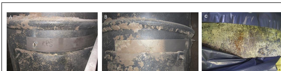
Figure 6-76. Images showing the shield sheet made of pre-oxidized Kanthal APMT material A) before exposure, B) after exposure from 2011-07-25 to 2011-12-05, and C) after exposure from 2011-07-25 to 2012-04-15 at Händelö plant.
