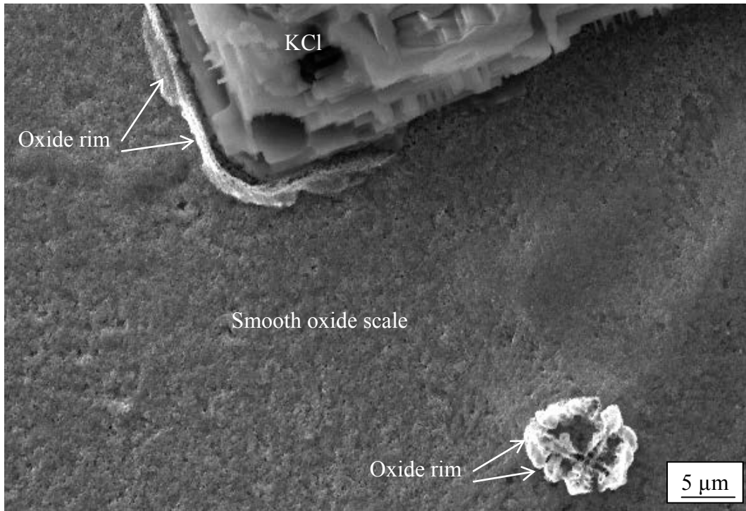
Figure 25: SEM SE image of the oxide scale and a KCl particle on pure Nickel after one hour of exposure, an oxide rim can be seen next to the KCl particle. The main part of the sample is covered with a smooth oxide scale.
