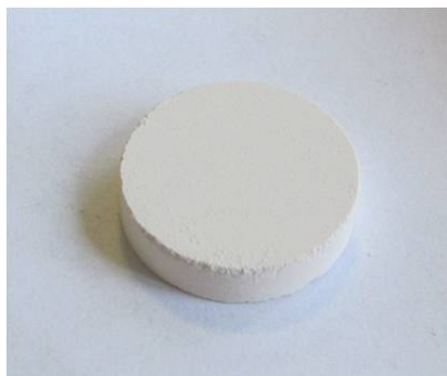
Figure 11: Pellet consisting of a mixture of KCl and oxide.
