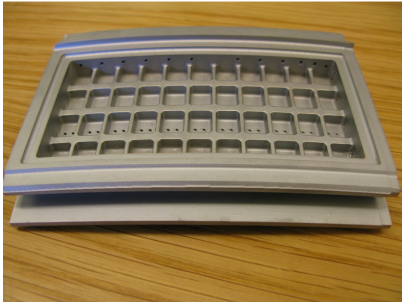
Fig. 1 The prototype of turbine heat shield manufactured with Cr10-ZrO 2 composite, the front side and back side of the prototype (15 x 7 x 3 cm).
