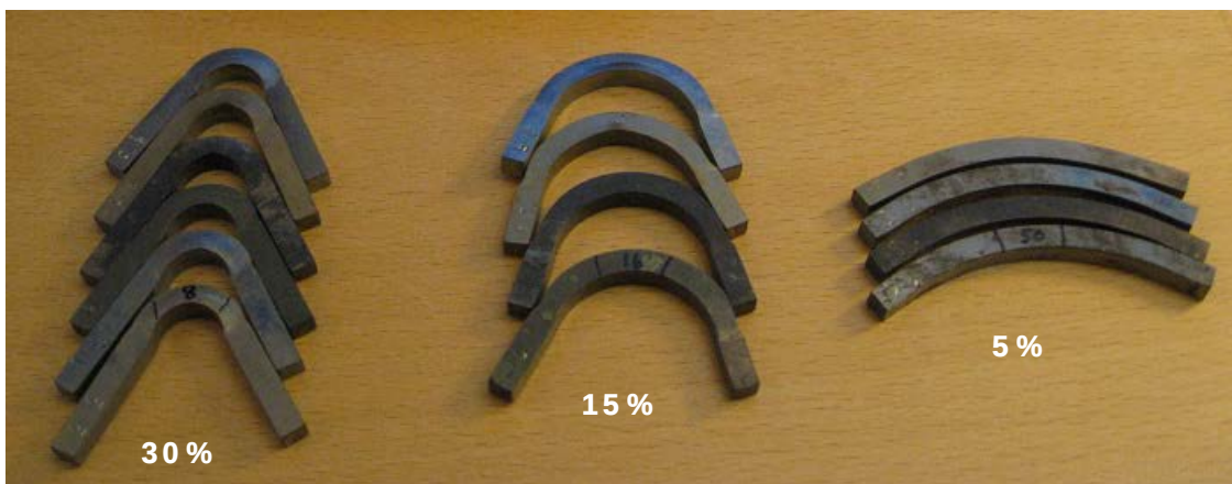
Figure 15. Bent samples exposed at 650°C for 24h.
