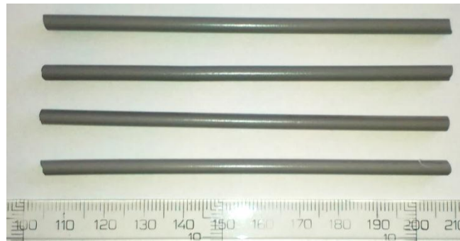
Fig.2 Pre-oxidized \text{MoSi}_2+15 \text{ vol.}\% \text{ZrO}_2 bars for flexure strength and K_{IC} testing. Notice that a glassy surface coating has been formed
