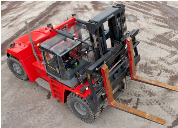
Kalmar heavy forklift with 18 tonnes lift capacity (Kalmar)
