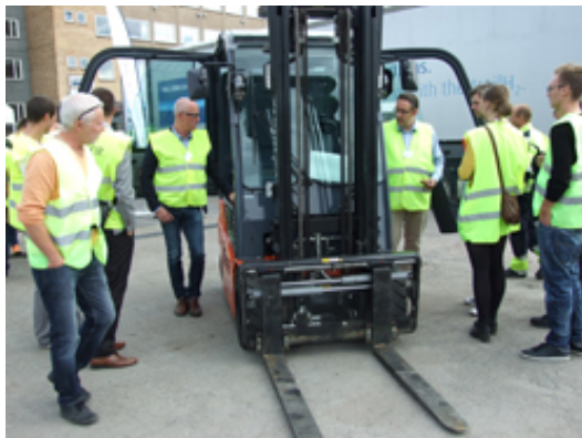
Toyota Fuel cell forklift, lift capacity 3 tonnes (Toyota material handling, 2015)
