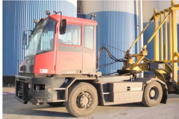
Kalmar terminal tractor with 105 tonnes load capacity (TFK)
