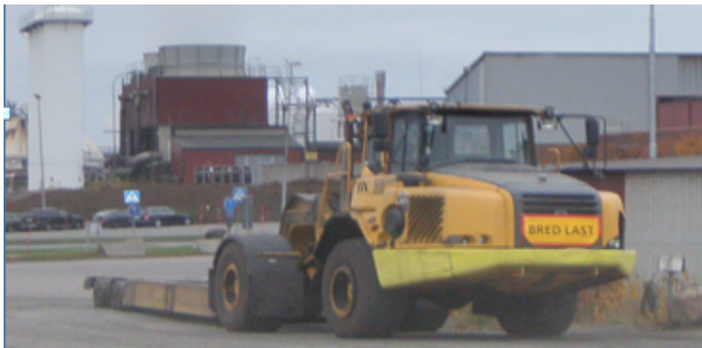
Volvo articulated tow tractor with load capacity of 60 tonnes (TFK)
