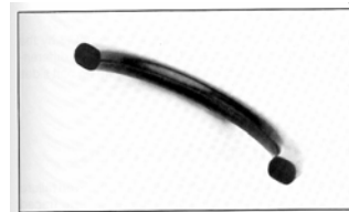
Fig. 9.9 Characteristic compression set. High deformation
