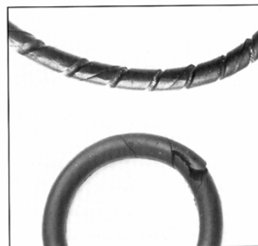
Fig. 9.10 and 9.11 Twisted O-ring with spiral marking, (9.10) or with spiral cuts in surface (9.11)
