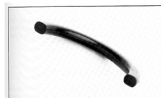
Fig. 9.9 Characteristic compression set. High deformation
