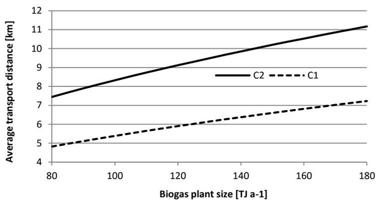
Figure 45. The average one-way transport distance between field and biogas plant depending on biogas plant size for the two regions. The biogas plant size is given as produced methane before losses.
