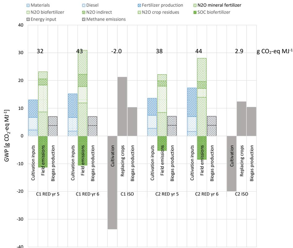
**Figure 14. Greenhouse gas emissions per MJ produced fuel. Net values are given above bars. Results according to EU RED compared to ISO-methodology. In addition to the differences in methodology, different input values are used in the EU RED calculations for some of the emissions (higher for electricity and diesel use, lower for mineral fertilizer production), and somewhat lower GWP characterization factors (see Appendix H & I for further details).**
