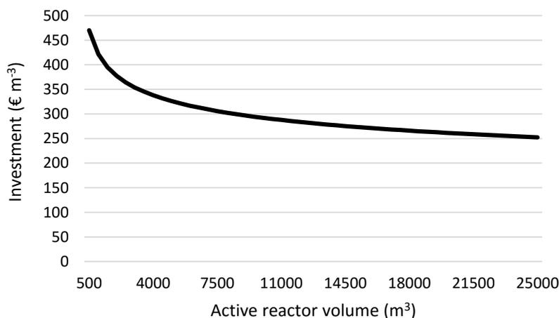
Figure 8. Calculated investment in biogas plant (Lantz, 2013).
