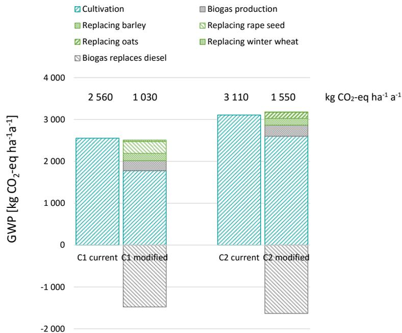
Figure 13. Greenhouse gas emissions after systems expansion. Net values are given above bars.
