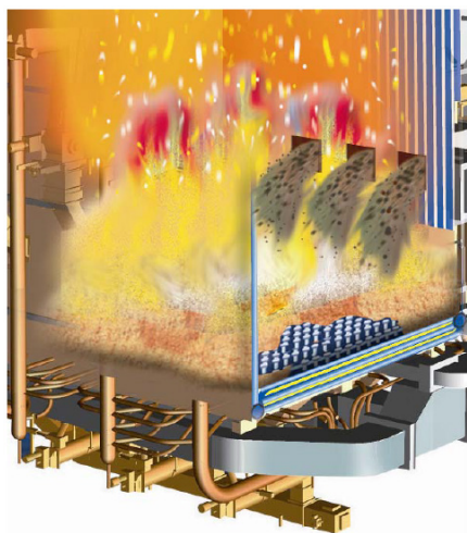
Figure 3 Bubbling fluidized bed boiler
