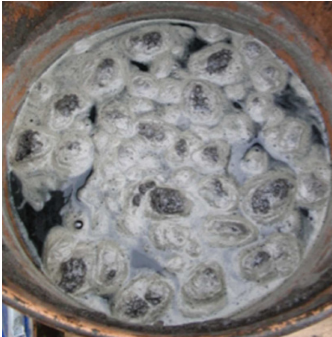
Figur 6-3 Biokolsslurry, producerad av bioslam Figure 6-3 Biocoal slurry, produced of biosludge
