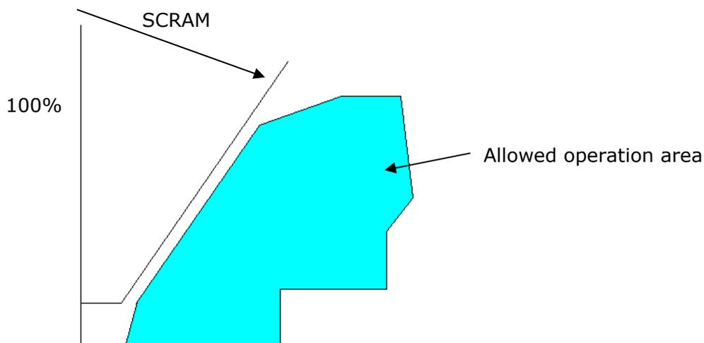
Fig. 9. Operation area, with reactor power as function of main coolant flow.
