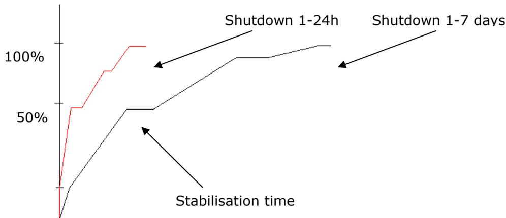
**Fig. 8. Start-up sequence, reactor power as function of time (arbitrary units). Note the difference in speed for the ramp-up in power.**
