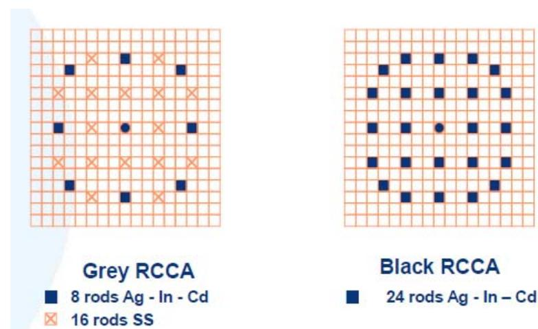
Fig. 15. Fuel assembly layout with typical design of grey and black RCCAs.
