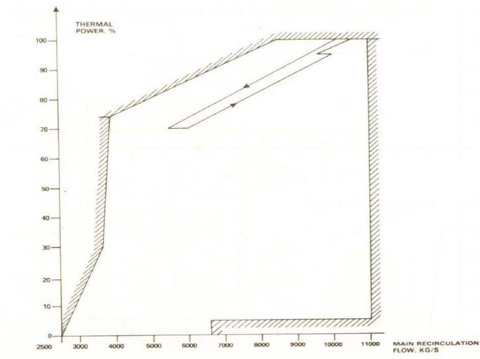
**Fig. 11. Schematic operating regime of a BWR. The arrows indicate a load swing down to 70 % power, see [22].**
