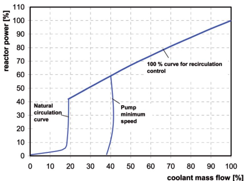
Fig. 6. Schematic characteristic curve for recirculation control (BWR) [3].
