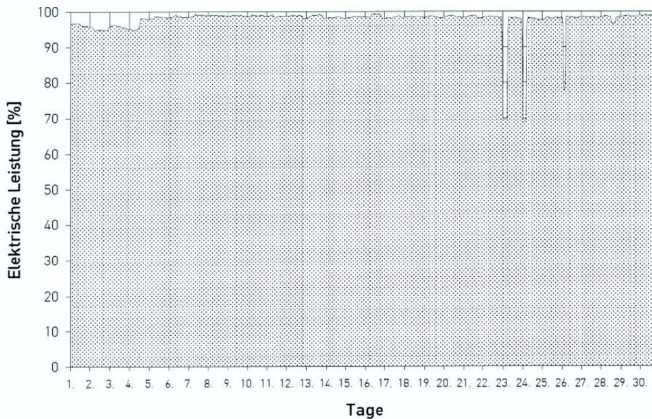
**Fig. 3. Power production (in % of rated power, 926 MW) for November 2009 at Philippsburg unit 1 (BWR).**
