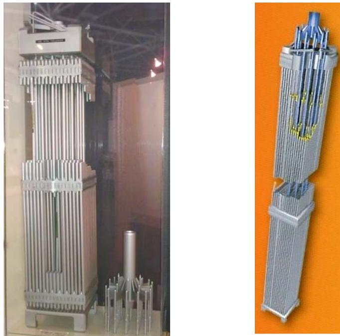
**Fig. 14. PWR fuel assembly (left) with the rod cluster control assembly (RCCA) handle and the 24 rods beside. RCCA (blue) inserted in fuel assembly (right).**
