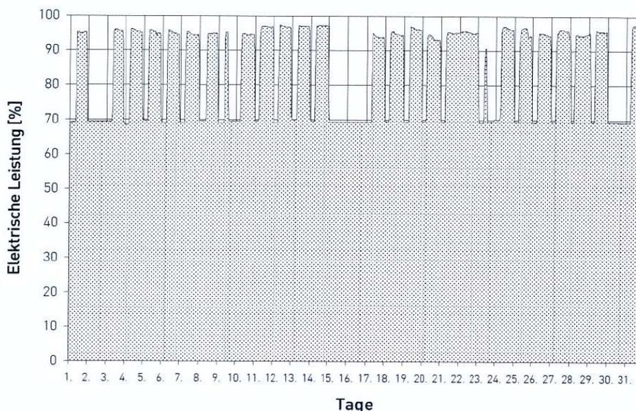
**Fig. 2. Power production (in % of rated power, 926 MW) for August 2009 at Philippsburg unit 1 (BWR).**
