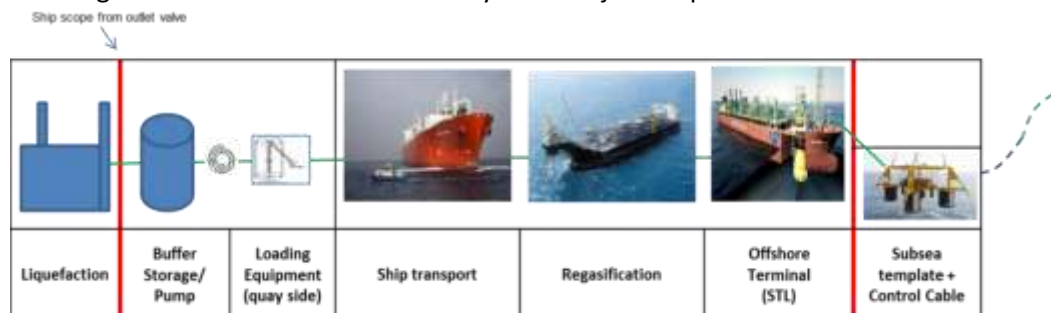
Figure 11 Ship transport system scope
