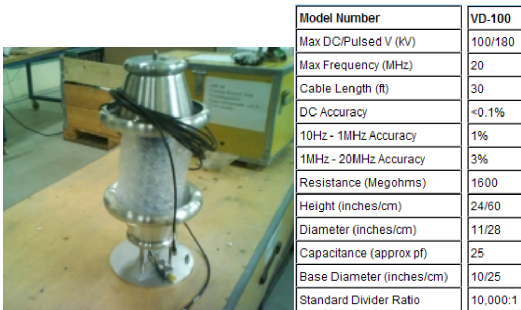
Figure 16: Voltage divider North Star Type VD-100 (photo left) and the parameters
